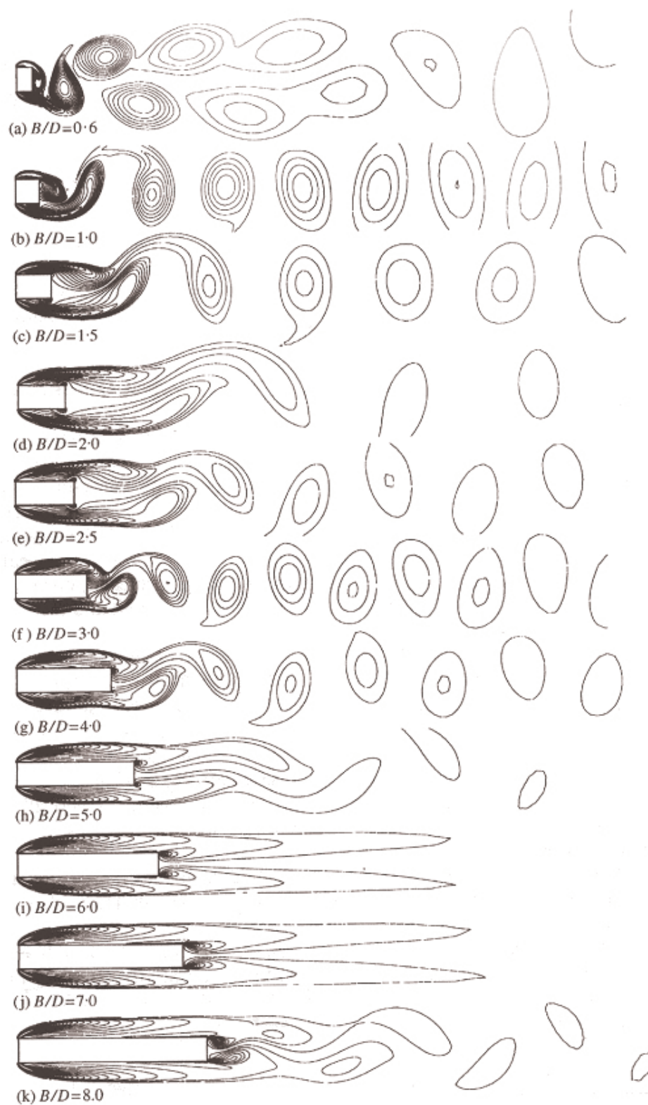
Figure 2-9: Instantaneous vorticity contours around rectangular cross-sections [Shimida et al. , 2002]
