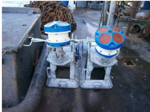
**Figure 5-3: Acoustic Current Doppler Profilers**
