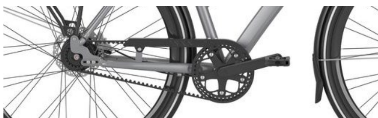
Belt drive and Shimano hub and brakes on a non-electric CityZen
