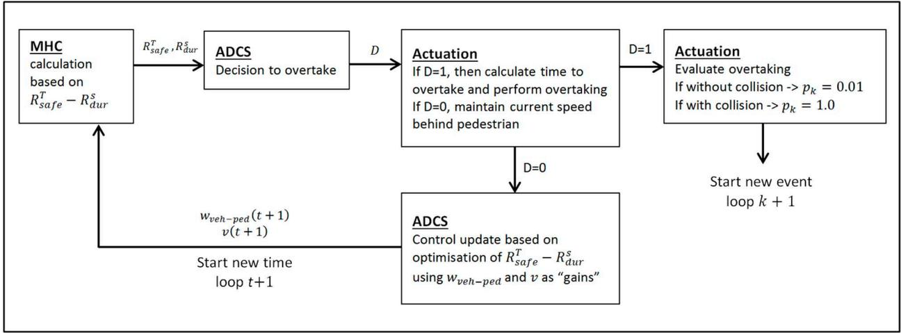
FIGURE 6. Implementation of control approach in the model.
