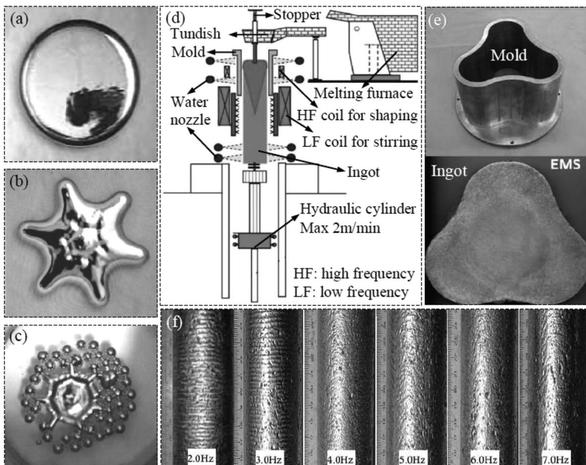
**Figure 4.** Electromagnetic effect on shaping of metallic materials a) mercury drop without EM effect; b) mercury drop is shaped by magnetic field with frequency of 2.1 Hz; c) gallium drop is emulsified by magnetic field with frequency of 6.2 Hz; d) equipment for the near-net shape continuous casting; e) mold of equipment shown in d) and the ingot; and f) products of soft-contact continuous casting under different electromagnetic field frequencies.<sup>[22]</sup>
