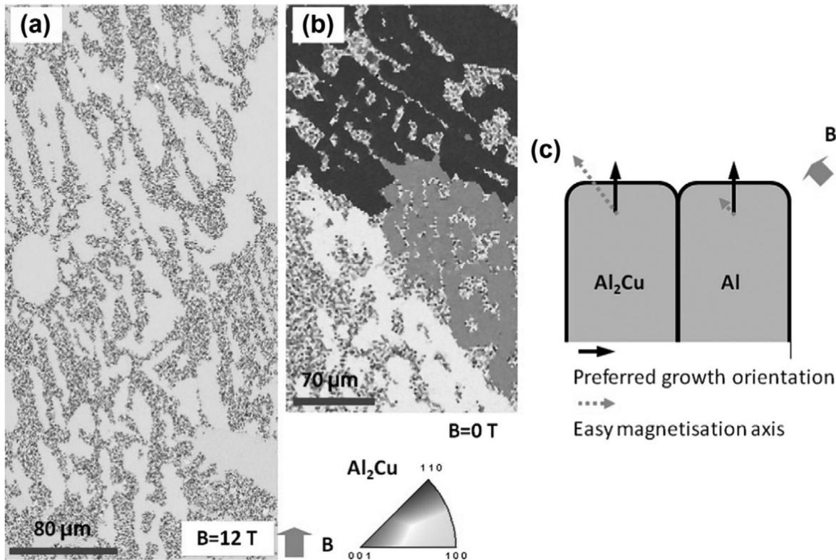
Figure 5. Strong magnetic field alignment of weakly magnetic metals.<sup>[43]</sup>
