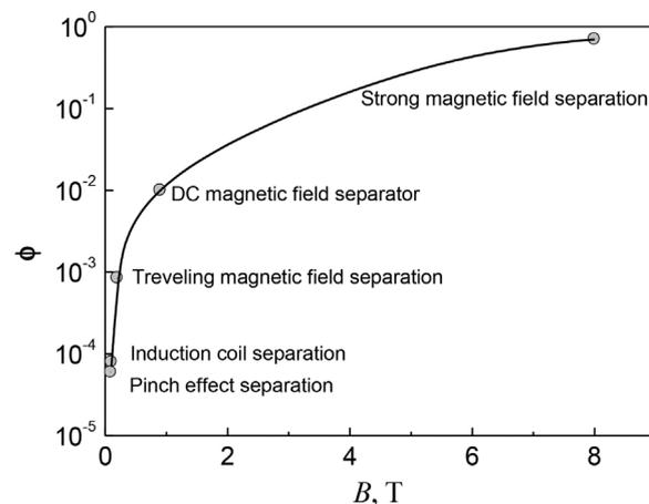
**Figure 7.** The energy coefficients ( $\phi$ ) versus magnetic flux density ( $B$ , T) of five representative separation technologies for inclusion removal from a liquid metal.
