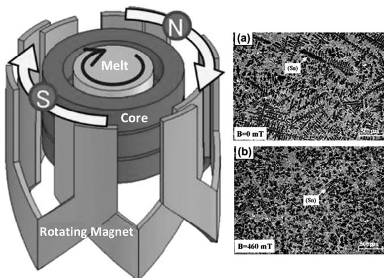
**Figure 2.** Effect of a rotating magnet on the solidification morphology of Bi–Sn alloys a) no magnet and b) with a magnet.<sup>[29]</sup>
