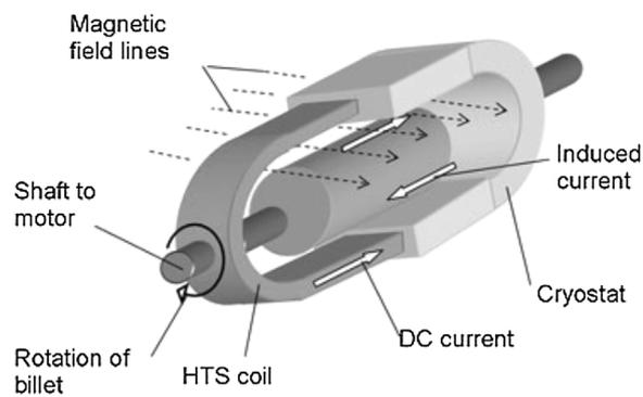
**Figure 3.** Induction heating of aluminum billet.<sup>[30]</sup>
