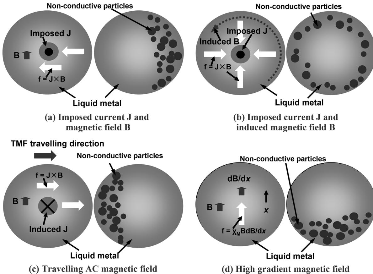
**Figure 6.** Different scenarios for inclusion removal from liquid metal using electromagnetic fields. a) direct electromagnetic field; b) alternative current; c) Traveling and alternative magnetic field (TMF); and d) High gradient magnetic field.<sup>[46]</sup>
