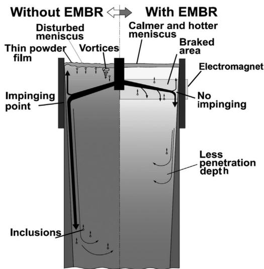
**Figure 1.** Effect of electromagnetic brakes (EMBR) on inclusion entrapment in steel during continuous casting<sup>[16]</sup> (color indicates different temperature).
