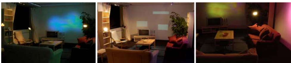
Fig. 3 Home living room lab with several projected atmospheres. Left picture a calm atmosphere (medium Warmth, low activity, medium attention), created by a subtly animated blue figure on the wall; Middle picture an active atmosphere, created by moving
