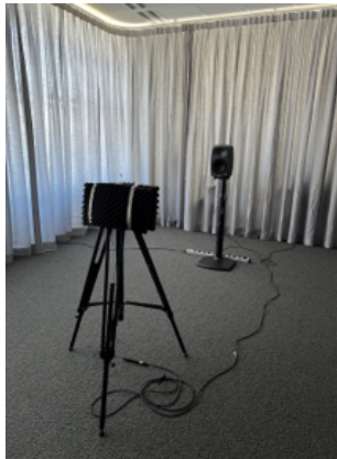
Figure 3.2: Acoustical and SNR measurement setup
