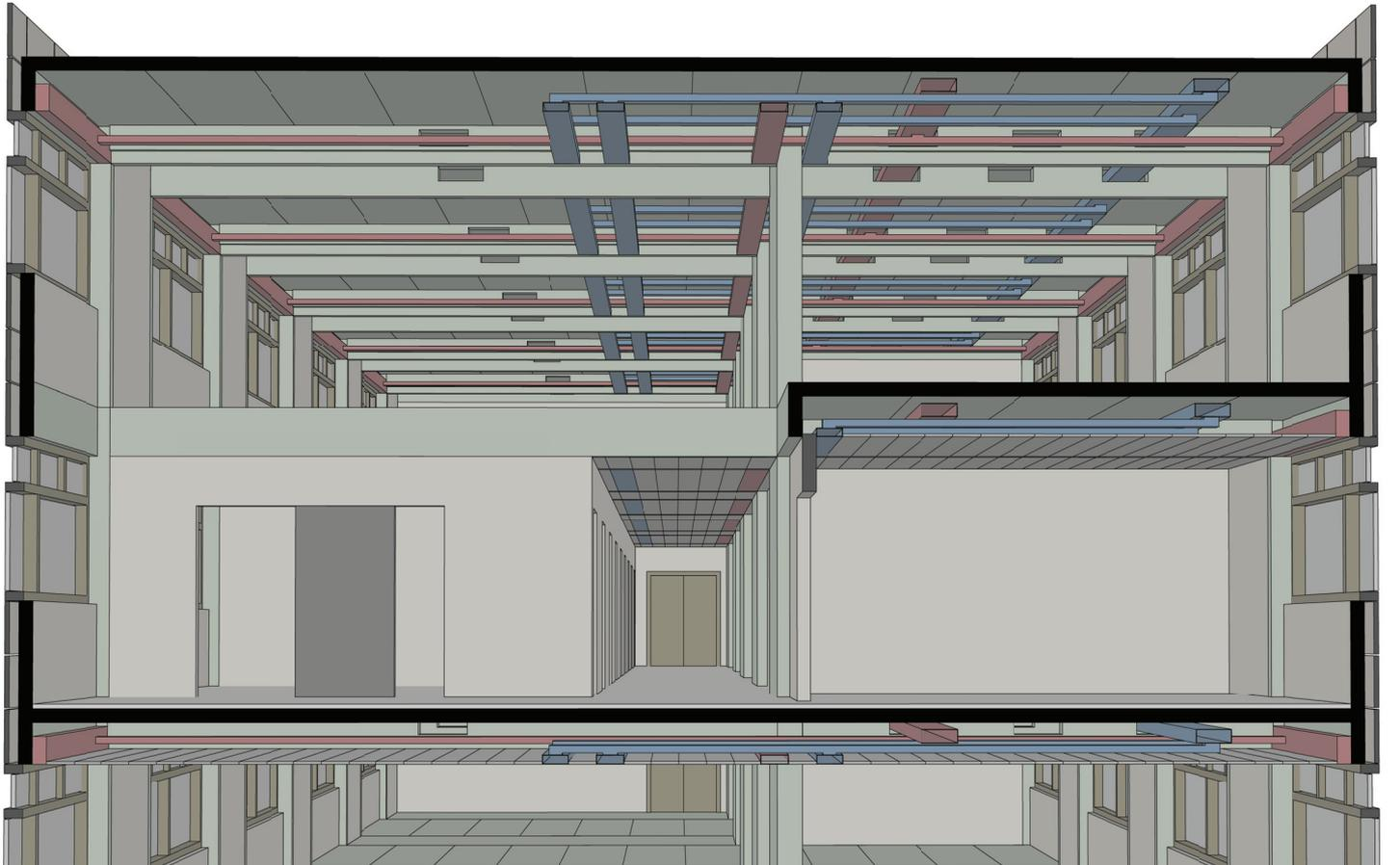
Typical cross section showing the integration of beams, floor slabs, ceiling panels, ducts and end user appliances
