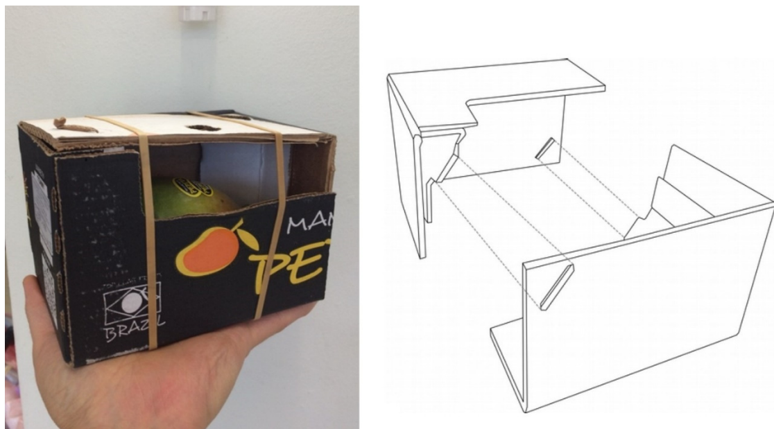
Figure 3. Design of a “Mango Equivalent Unit” (MEU).
