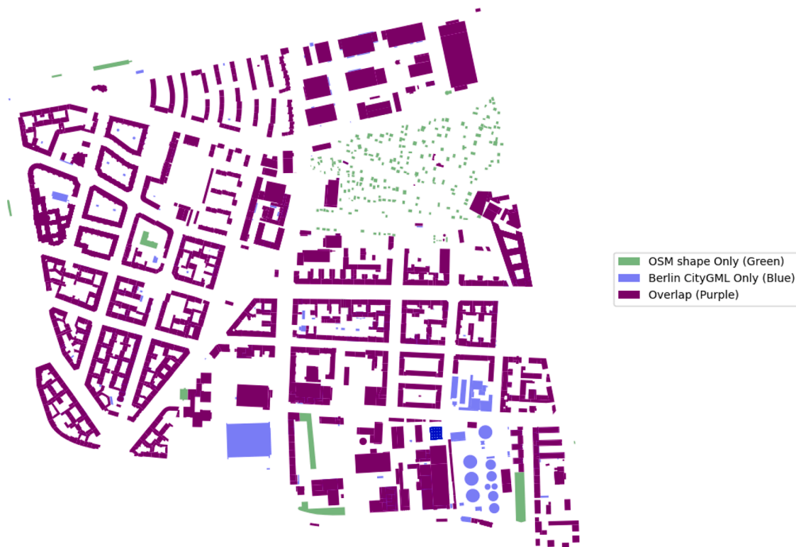
Fig. 5. Comparison of the geometric input data for CityGML and OSM. Although both input formats contain most buildings, OSM contains more up-to-date data as well as smaller, non-permanent buildings (sheds).
