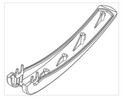
Figure 50. Design choice representation of optimized armrest for internal ribs.
