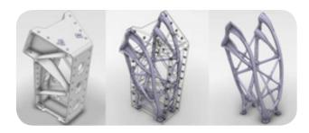
Last, EADS Innovations Works uses DMLS printing of EOS to manufacture titanium replacement parts of a previously cast steel nacelle hinge bracket on an Airbus A320. This optimization saved 10kg per set which comes down to a 75% reduction in raw material consumption (Warwick G., 2013).
