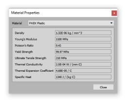
Figure 43. Material proposition of PAEK from software Fusion360.
