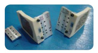
At last, a fitting alignment tool which was previously made out of metal, being very heavy and difficult to handle, which is now made of plastic. This resulted in 70% of labor savings due to the fact it was sufficient light so one single engineer could operate it. And in addition 90% cost reduction has been achieved (Schiller G.J., 2015).
