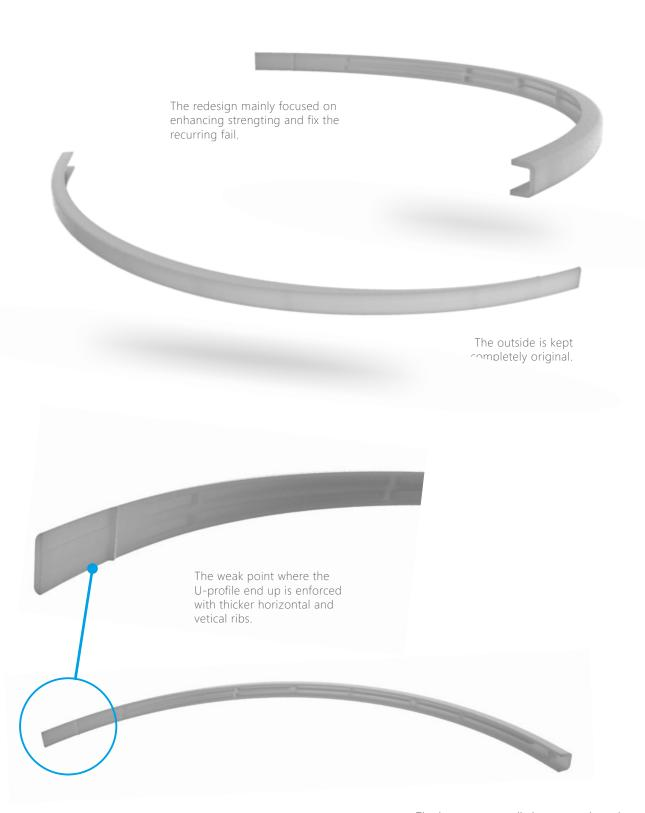
The bumper normally has a metal coating. This post-process should likewise applied on the redesign to maintain the same business class cabin appearance.
