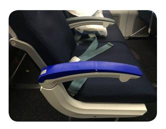
Figure 65. Picture of first prototype tested on fit and dimensions in the 787-9 cabin.
