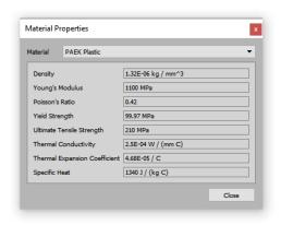
Figure 41. Material proposition of PAEK from software Fusion360.
