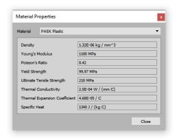
Figure 39. Material proposition of PAEK from software Fusion360.
