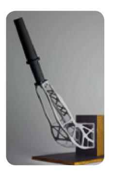
Moreover, a new bracket has been designed and manufactured for the next Eurostar E3000 satellite. This new topology optimized aluminum bracket integrates 44 rivets and parts into 1 single part. Reducing the weight by 35% while increasing the stiffness up to 40% (Shapiro A.A. et al., 2016).
