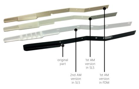
Figure 34. A picture of the original, SLS and FDM printed part Tolga Inan has developed.
