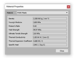
Figure 37. Material proposition of PAEK from software Fusion360.
