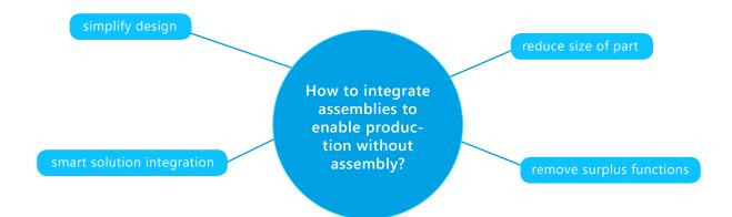
The mindmap created for the toilet roll holder is mainly focusing integrating assemblies which would enable to produce the complete assembly as one single part. This could be done in multiple ways like mentioned in the mindmap, but simply be done by redesigning the component for AM by stitching the seperate parts together making it one piece. Even functional parts like springs could be printed with AM enabling the integrationg of smart solutions.
