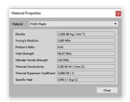
Figure 45. Material proposition of PAEK from software Fusion360.
