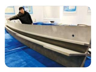
Lockheed Martin collaborated with Sciaky, an industry-leading EBM process expert. Together they fabricated a wing spar for the Lockheed Martin F-35 and wing leading edges for the Dassault Falcon 5X (Trimble S., 2014).
