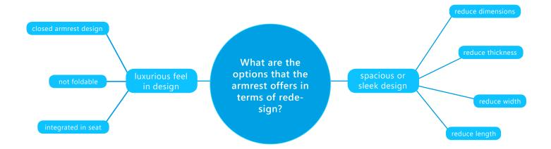
A rather fast and simple mindmap is carried out in order to write down thoughts for ideation. The Zodiac seat armrest has been chosen to enhance its current lead time. However, lead time is not directly or only design related. Substituting only the production method by AM could lead to reaching the goal. Nevertheless, the mind map has been used to find redesign possibilities for this component.
