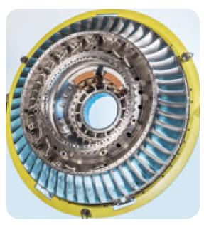
Pratt and Whitney 3D prints compressor stators and sync ring brackets for their PW1500G engines. These engines are used on Bombardier CSeries passenger aircrafts. AM helped saving 15 months in lead time and up to 50% in weight in a single part (Peach M., 2015).
