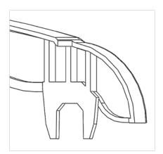
Figure 52. Design choice representation of optimized armrest ribs for u-shaped clips.
