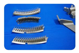
NASA manufactures nickel-chromium alloy rocket injector parts for the J-2X engines using the SLM process. The costs are reduced by 35% while increasing the lead time and integrating the assembly from 115 parts to 2 in total. This integration and reduction of parts and connections made the injector structurally stronger and more reliable leading to the overall safety (Szondy D., 2012; Zhou F. et al., 2014).
