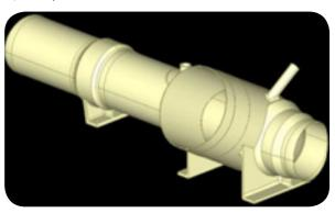
There are about 100 AM parts used for the air cooling ducts in the Super Hornet jets (Khajavi S.H. et al., 2014).
