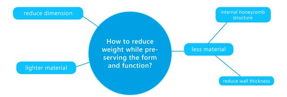
A rather fast and simple mindmap is carried out with the aim of solidifying what has been built up with experience in terms of knowledge. The mind map only focuses on how to reduce weight while the bi-fold table has a lot more potential for handling the other AM benefits. This has been chosen as reducing weight is the main focus why this component has been chosen.
