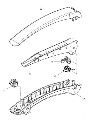
Figure 63. Assembly of the original Zodiac seat armrest.
