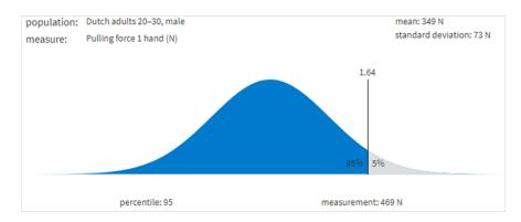
Figure 44. Result of DINED pulling force with one hand P95 male, 20-30 age.
