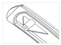
Figure 51. Design choice representation of optimized armrest for screw pin ribs
