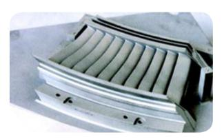
Rolls Royce 3D prints the front bearing housing, holding 48 aerofoils of their Trent-XWB 97 engine. This is the largest engine part printed in titanium making use of Electron Beam Melting (EBM). Using AM reduced the lead time by 30% compared to conventional manufacturing methods. The Trent-XWB is the sole engine type for the Airbus A350 (Anderson S. 2015; Morrison M., 2015).
