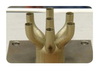
TWI additively manufactured a thin-walled helicopter engine combustion chamber using a five axis LMD process without support mechanisms. The build time was reduced from months to just 7.5 hours (T. Ltd., 2014).
