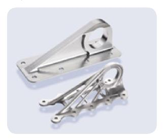
For another satellite, the Sentinel-1 Earth-observation satellite, is this time an antenna support developed and printed in aluminum-silicate-magnesium alloy by selective laser sintering (SLS). This created a lightweight parts enabling a mass reduction of 56% (Raviv D. et al., 2014).
