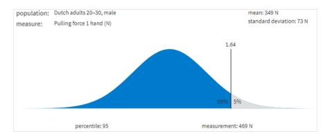
Figure 42. Result of DINED pulling force with one hand P95 male, 20-30 age.
