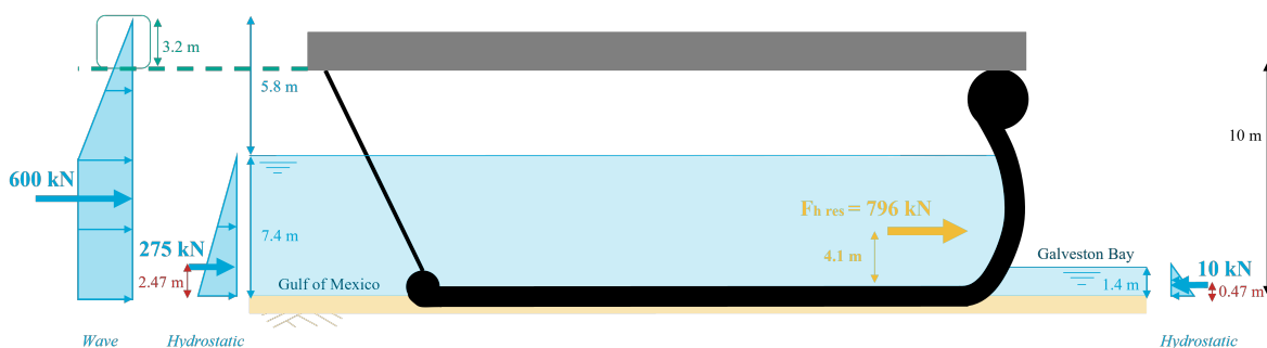
Figure H.5: Geometric horizontal forces on flexible membrane fabric
