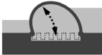
Figure C.6: Cross-section of inflatable gate (L. F. Mooyaart and Jonkman, 2017)
