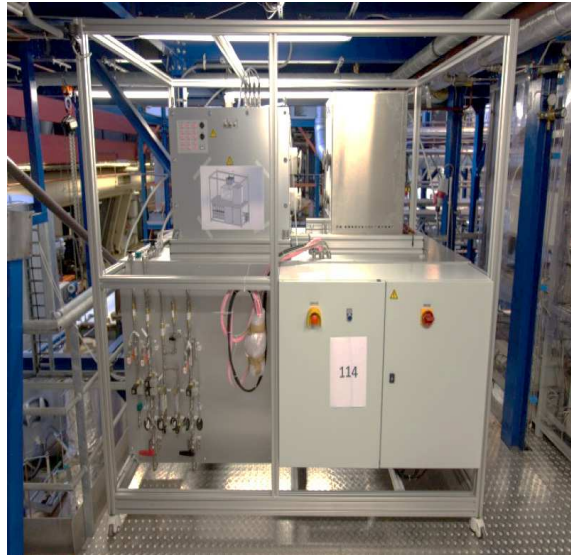
Figure 1. 4 kW SOFC power plant designed for gasifier integration at TU Delft.
