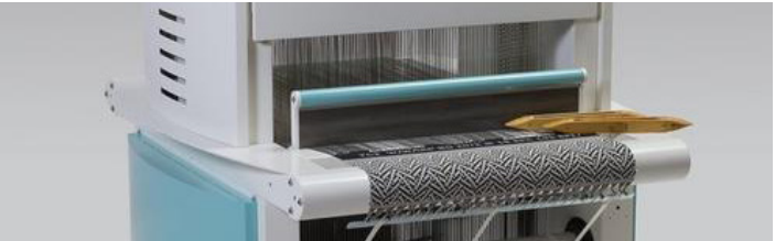
Figure 18: Jacquard loom TC2 (2012) (Engineering, n.d.-b).
