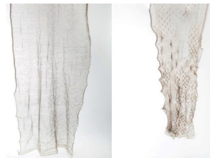
Figure 24: On the left, the textile is shown before being sprayed with cold water, and on the right, after being sprayed with cold water (Scott, 2018).
