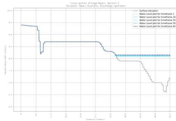
**Figure F.64:** Cross section of the NEW situation of section 5 in the Lage Raam | Scenario: Discharge  $T > 1X25$  year
