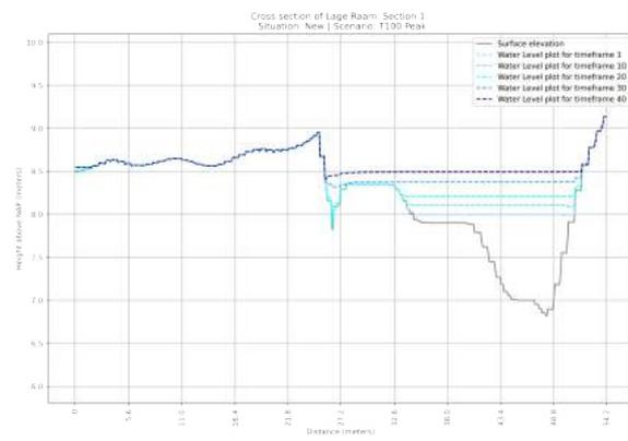
**Figure 10.18:** Cross section of the NEW situation of section 1 in the Lage Raam | Scenario: T=1x100 year Peak Rainfall event
