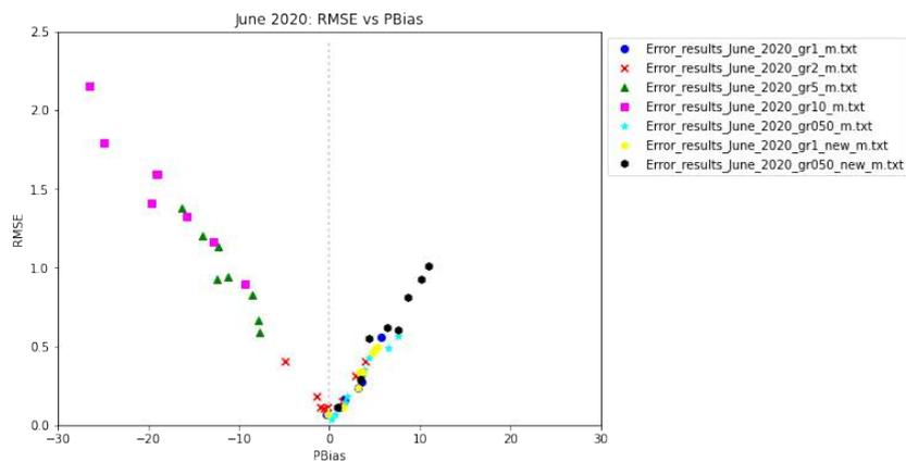
**Figure 10.4:** RMSE vs PBIAs for June 2020 scenario, each simulation run with different grid cell sizes (gr)
