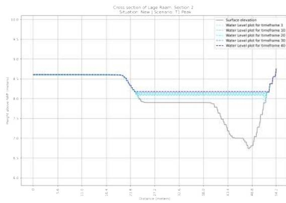
**Figure F.18:** Cross section of the NEW situation of section 2 in the Lage Raam | Scenario:  $T=1x1$  year Peak Rainfall event
