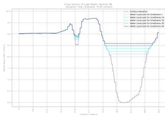
**Figure F.59:** Cross section of the OLD situation of section 4b in the Lage Raam | Scenario: T=1x100 year Uniform Rainfall event
