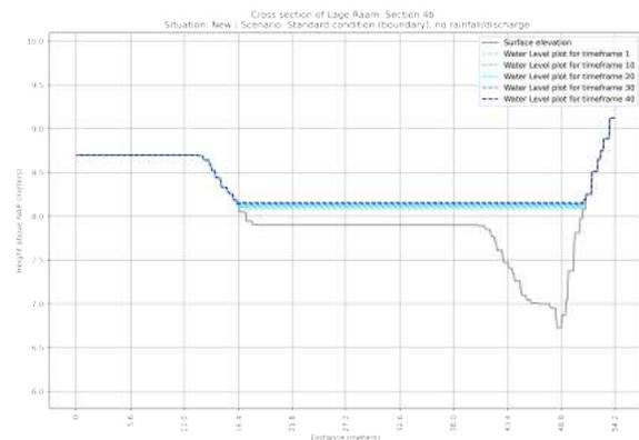
**Figure F.50:** Cross section of the NEW situation of section 4b in the Lage Raam | Scenario: Standard situation
