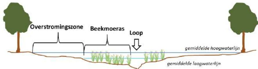
Figure 2.1: Swamp streams cross section example by STOWA
