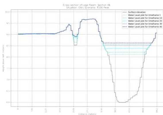
**Figure F.55:** Cross section of the OLD situation of section 4b in the Lage Raam | Scenario:  $T=1x100$  year Peak Rainfall event
