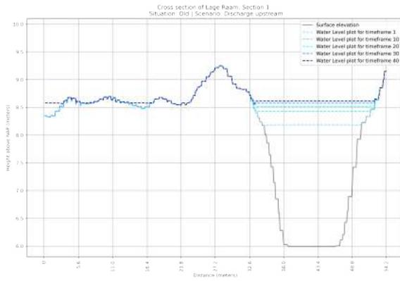
**Figure F.3:** Cross section of the OLD situation of section 1 in the Lage Raam | Scenario: Discharge  $T > 1X25$  year
