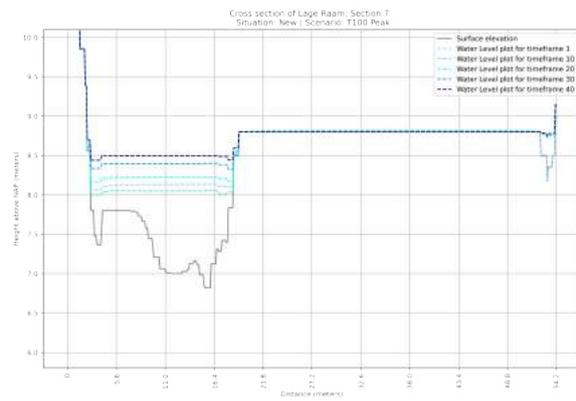
**Figure F.92:** Cross section of the NEW situation of section 7 in the Lage Raam | Scenario:  $T=1x100$  year Peak Rainfall event
