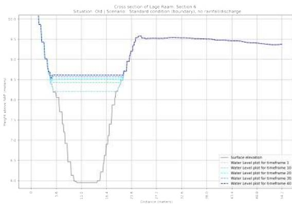
**Figure F.73:** Cross section of the OLD situation of section 6 in the Lage Raam | Scenario: Standard situation
