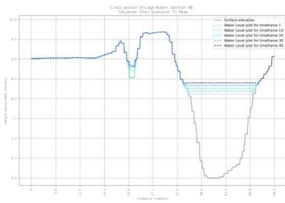
**Figure F.53:** Cross section of the OLD situation of section 4b in the Lage Raam | Scenario:  $T=1x1$  year Peak Rainfall event
