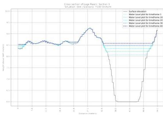
**Figure F.11:** Cross section of the OLD situation of section 1 in the Lage Raam | Scenario: T=1x100 year Uniform Rainfall event
