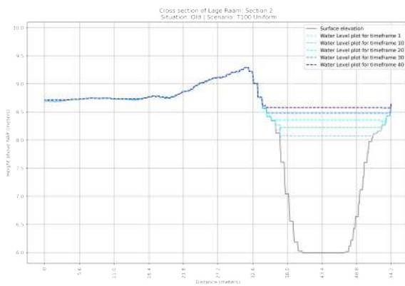
**Figure F.23:** Cross section of the OLD situation of section 2 in the Lage Raam | Scenario: T=1x100 year Uniform Rainfall event
