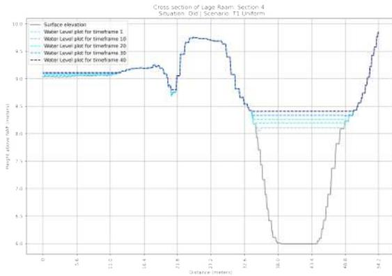
**Figure F.45:** Cross section of the OLD situation of section 4 in the Lage Raam | Scenario: T=1x1 year Uniform Rainfall event
