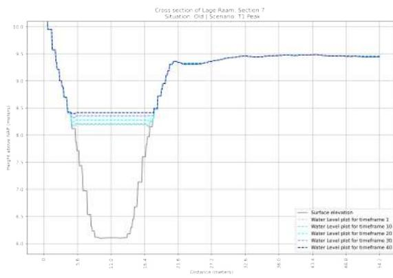
**Figure F.89:** Cross section of the OLD situation of section 7 in the Lage Raam | Scenario:  $T=1x1$  year Peak Rainfall event
