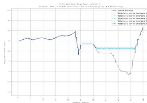
**Figure F.2:** Cross section of the NEW situation of section 1 in the Lage Raam | Scenario: Standard situation
