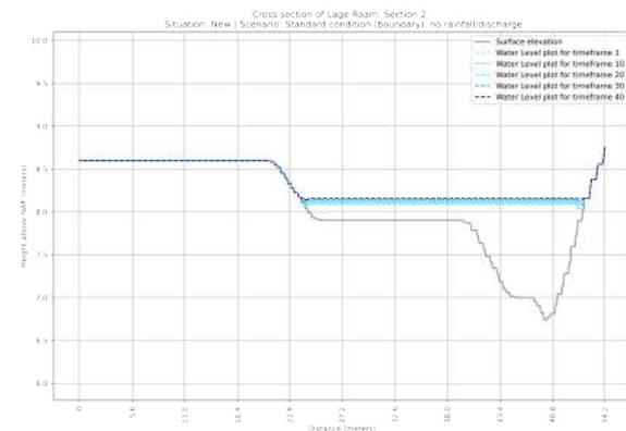
**Figure F.14:** Cross section of the NEW situation of section 2 in the Lage Raam | Scenario: Standard situation
