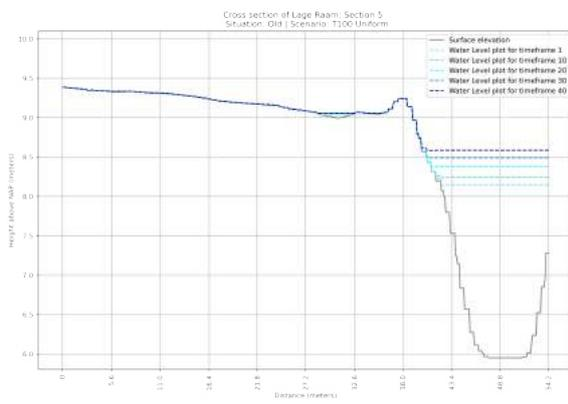
**Figure F.71:** Cross section of the OLD situation of section 5 in the Lage Raam | Scenario: T=1x100 year Uniform Rainfall event
