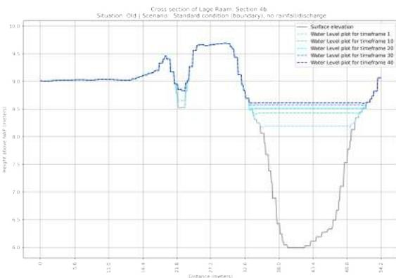
**Figure F.49:** Cross section of the OLD situation of section 4b in the Lage Raam | Scenario: Standard situation
