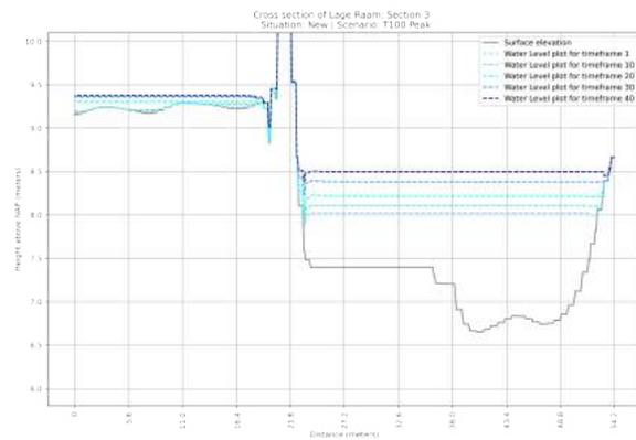
**Figure F.32:** Cross section of the NEW situation of section 3 in the Lage Raam | Scenario:  $T=1x100$  year Peak Rainfall event
