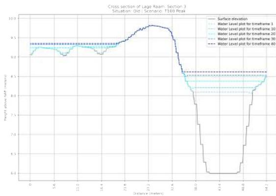
**Figure F.31:** Cross section of the OLD situation of section 3 in the Lage Raam | Scenario:  $T=1x100$  year Peak Rainfall event
