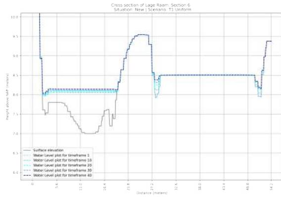
**Figure F.82:** Cross section of the NEW situation of section 6 in the Lage Raam | Scenario: T=1x1 year Uniform Rainfall event
