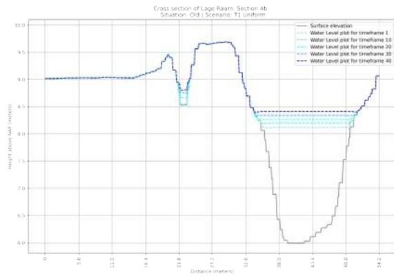
**Figure F.57:** Cross section of the OLD situation of section 4b in the Lage Raam | Scenario: T=1x1 year Uniform Rainfall event
