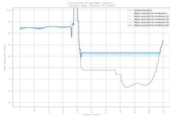
**Figure F.34:** Cross section of the NEW situation of section 3 in the Lage Raam | Scenario: T=1x1 year Uniform Rainfall event
