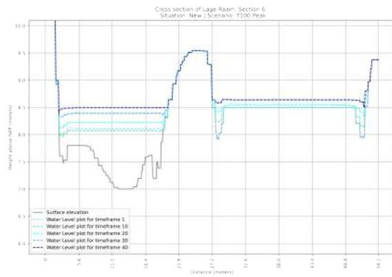
**Figure F.80:** Cross section of the NEW situation of section 6 in the Lage Raam | Scenario:  $T=1x100$  year Peak Rainfall event
