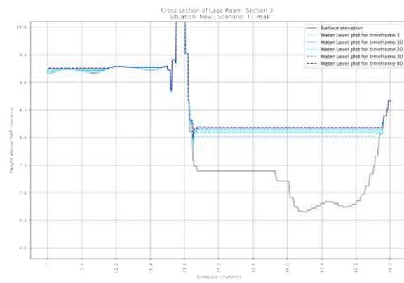
**Figure F.30:** Cross section of the NEW situation of section 3 in the Lage Raam | Scenario:  $T=1x1$  year Peak Rainfall event
