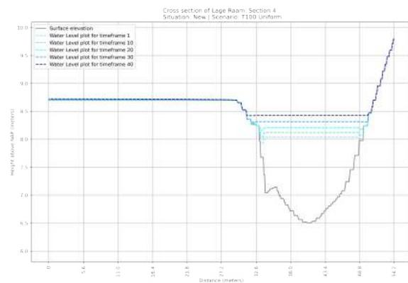
**Figure F.48:** Cross section of the NEW situation of section 4 in the Lage Raam | Scenario: T=1x100 year Uniform Rainfall event
