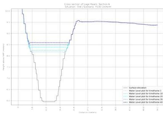
**Figure F.83:** Cross section of the OLD situation of section 6 in the Lage Raam | Scenario: T=1x100 year Uniform Rainfall event
