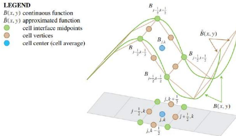
Figure A.4: Visualisation of 2D piecewise linearization (Bollermann et al., 2014)
