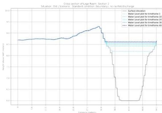
**Figure F.13:** Cross section of the OLD situation of section 2 in the Lage Raam | Scenario: Standard situation
