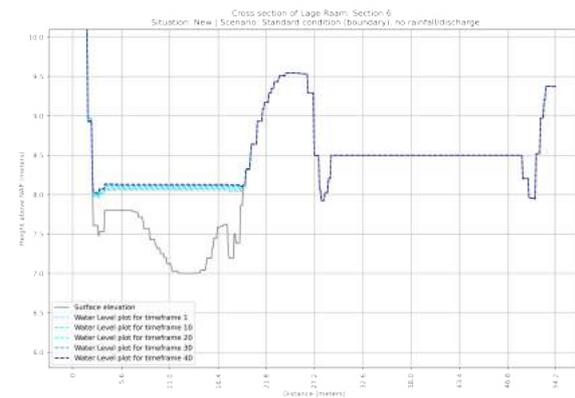
**Figure F.74:** Cross section of the NEW situation of section 6 in the Lage Raam | Scenario: Standard situation
