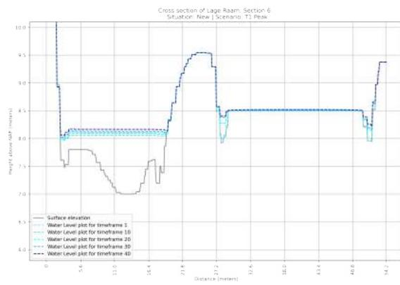
**Figure F.78:** Cross section of the NEW situation of section 6 in the Lage Raam | Scenario:  $T=1x1$  year Peak Rainfall event
