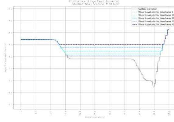
**Figure F.56:** Cross section of the NEW situation of section 4b in the Lage Raam | Scenario:  $T=1x100$  year Peak Rainfall event
