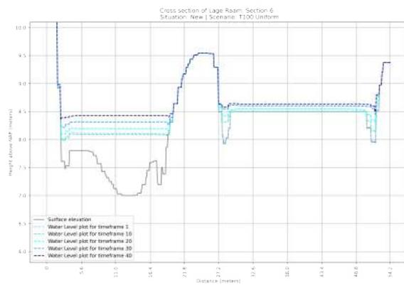
**Figure F.84:** Cross section of the NEW situation of section 6 in the Lage Raam | Scenario: T=1x100 year Uniform Rainfall event
