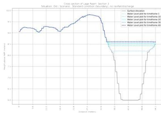
**Figure F.25:** Cross section of the OLD situation of section 3 in the Lage Raam | Scenario: Standard situation
