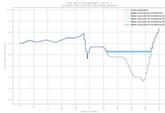
**Figure 10.16:** Cross section of the NEW situation of section 1 in the Lage Raam | Scenario: Discharge T > 1X25 year
