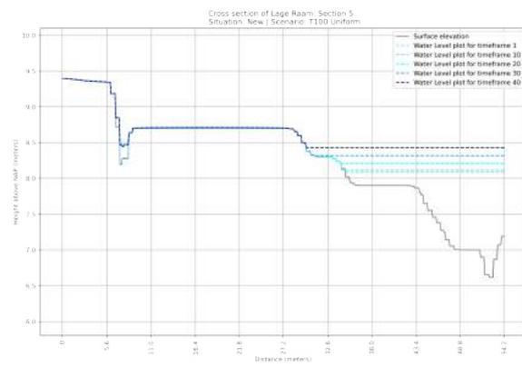
**Figure F.72:** Cross section of the NEW situation of section 5 in the Lage Raam | Scenario: T=1x100 year Uniform Rainfall event
