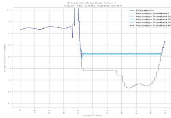
**Figure F.28:** Cross section of the NEW situation of section 3 in the Lage Raam | Scenario: Discharge  $T > 1X25$  year
