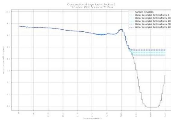
**Figure F.65:** Cross section of the OLD situation of section 5 in the Lage Raam | Scenario:  $T=1x1$  year Peak Rainfall event
