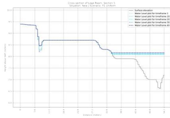
**Figure F.70:** Cross section of the NEW situation of section 5 in the Lage Raam | Scenario: T=1x1 year Uniform Rainfall event
