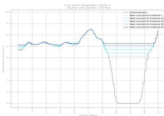
**Figure 10.17:** Cross section of the OLD situation of section 1 in the Lage Raam | Scenario: T=1x100 year Peak Rainfall event
