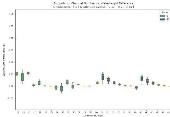
**Figure C.17:** Boxplot for grid placement results divided per channel and angle. Small grid cell sizes (0.11 to 0.25 meters)
