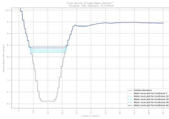
**Figure F.93:** Cross section of the OLD situation of section 7 in the Lage Raam | Scenario: T=1x1 year Uniform Rainfall event
