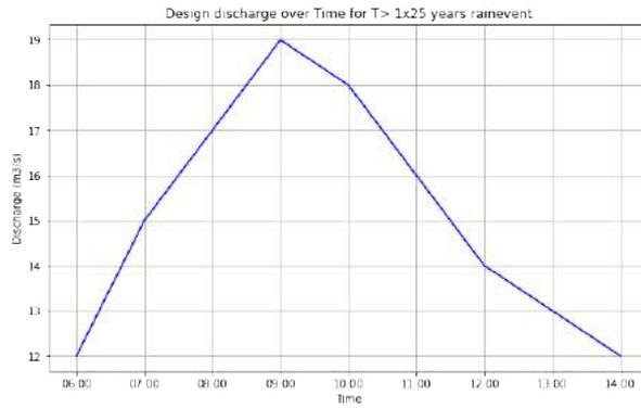
**Figure 9.5:** Hydrograph discharge design for T>1x25
