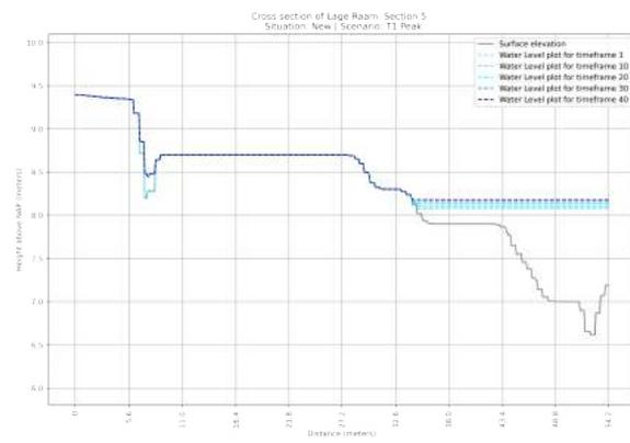
**Figure F.66:** Cross section of the NEW situation of section 5 in the Lage Raam | Scenario:  $T=1x1$  year Peak Rainfall event
