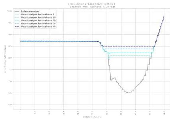
**Figure F.44:** Cross section of the NEW situation of section 4 in the Lage Raam | Scenario:  $T=1x100$  year Peak Rainfall event
