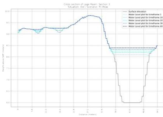
**Figure F.29:** Cross section of the OLD situation of section 3 in the Lage Raam | Scenario:  $T=1x1$  year Peak Rainfall event
