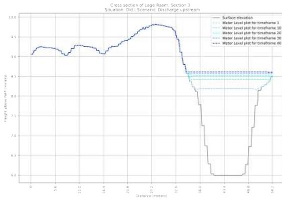
**Figure F.27:** Cross section of the OLD situation of section 3 in the Lage Raam | Scenario: Discharge  $T > 1X25$  year
