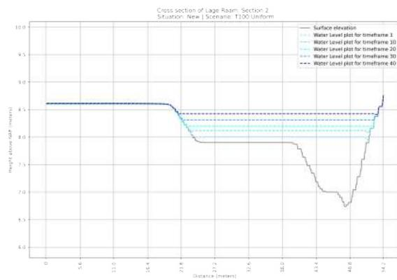
**Figure F.24:** Cross section of the NEW situation of section 2 in the Lage Raam | Scenario: T=1x100 year Uniform Rainfall event
