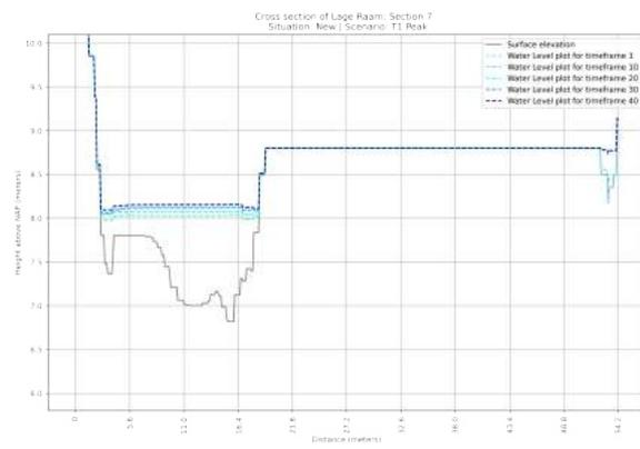
**Figure F.90:** Cross section of the NEW situation of section 7 in the Lage Raam | Scenario:  $T=1x1$  year Peak Rainfall event
