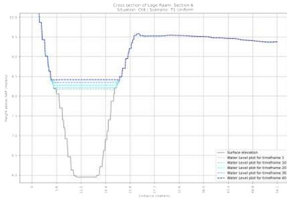
**Figure F.81:** Cross section of the OLD situation of section 6 in the Lage Raam | Scenario: T=1x1 year Uniform Rainfall event
