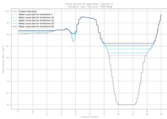
**Figure F.43:** Cross section of the OLD situation of section 4 in the Lage Raam | Scenario:  $T=1x100$  year Peak Rainfall event
