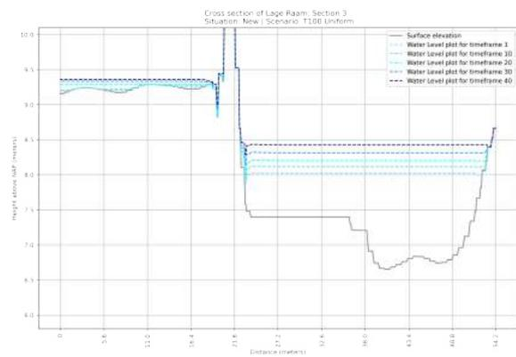
**Figure F.36:** Cross section of the NEW situation of section 3 in the Lage Raam | Scenario: T=1x100 year Uniform Rainfall event
