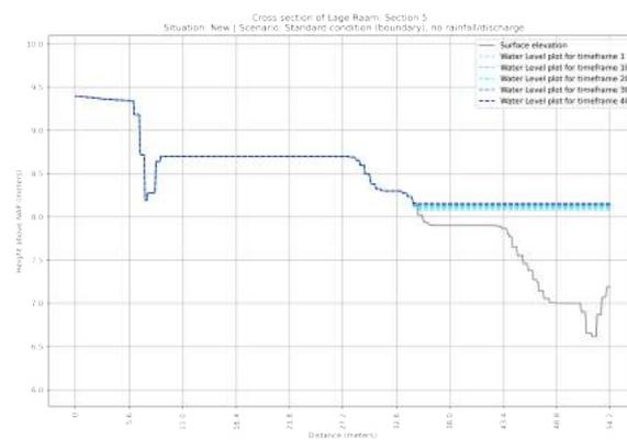
**Figure F.62:** Cross section of the NEW situation of section 5 in the Lage Raam | Scenario: Standard situation
