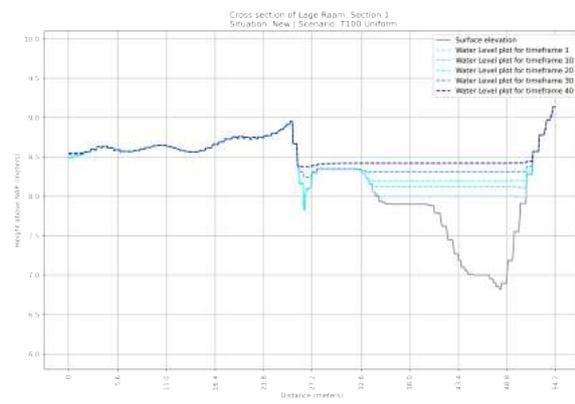
**Figure F.12:** Cross section of the NEW situation of section 1 in the Lage Raam | Scenario: T=1x100 year Uniform Rainfall event
