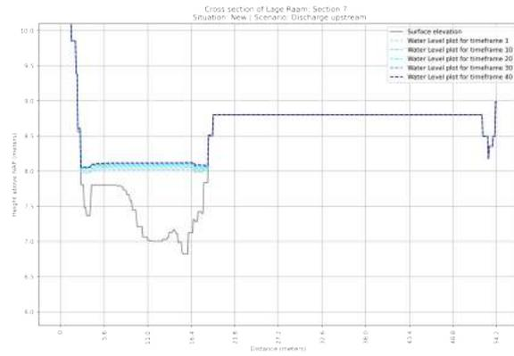
**Figure F.88:** Cross section of the NEW situation of section 7 in the Lage Raam | Scenario: Discharge  $T > 1X25$  year
