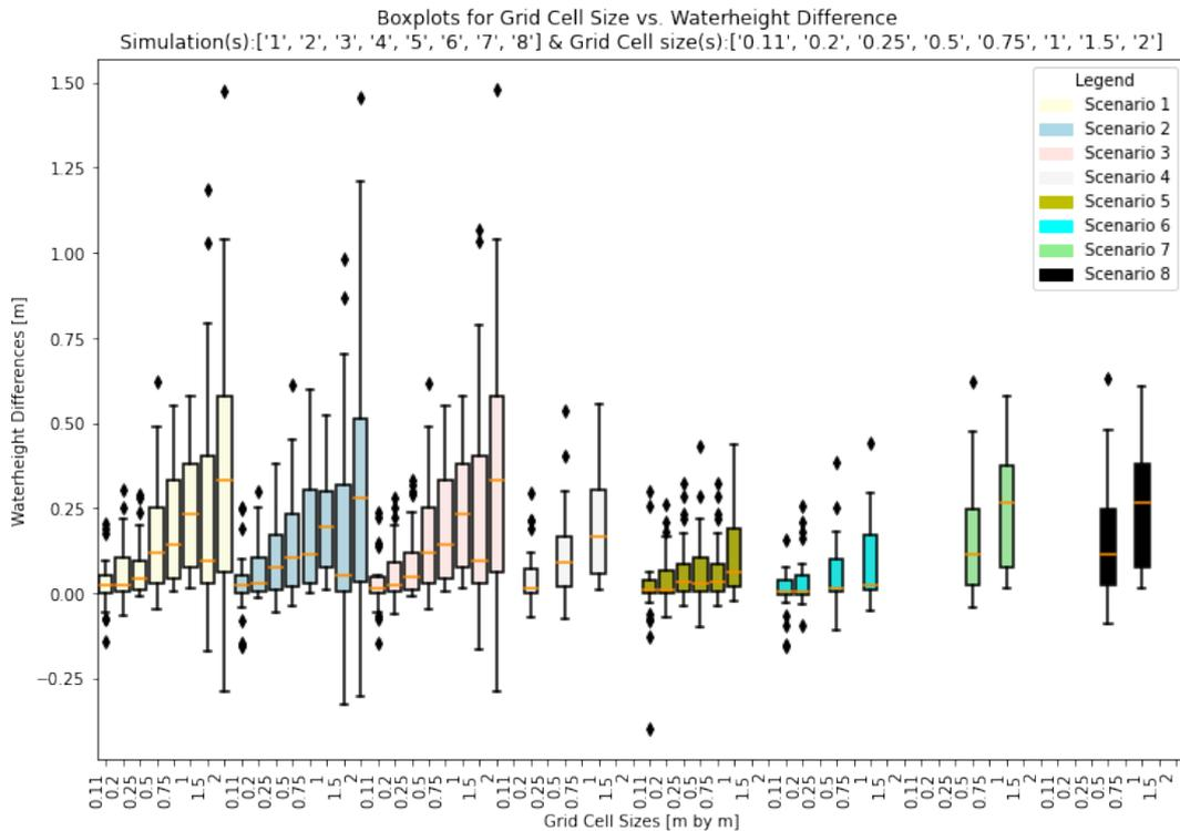
**Figure 5.12:** All Results of simulations on grid cell sizes and their according scenarios
