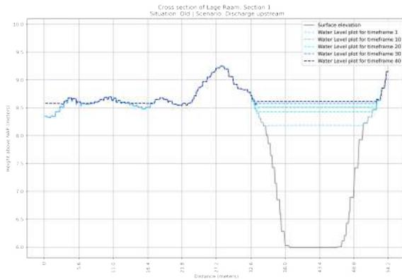
**Figure 10.15:** Cross section of the OLD situation of section 1 in the Lage Raam | Scenario: Discharge T > 1X25 year
