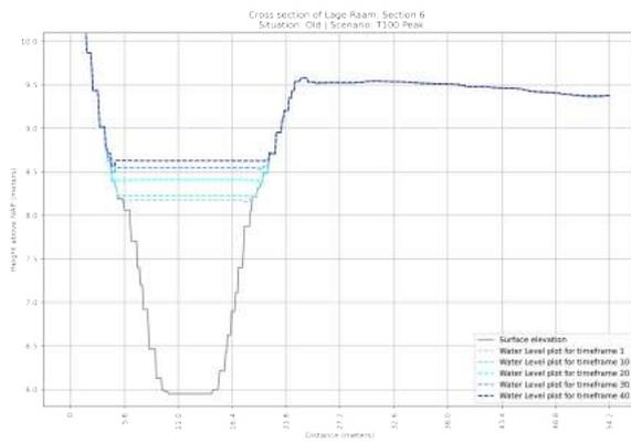
**Figure F.79:** Cross section of the OLD situation of section 6 in the Lage Raam | Scenario:  $T=1x100$  year Peak Rainfall event
