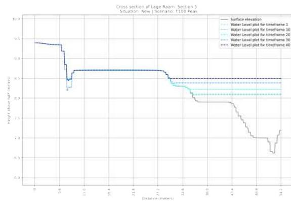
**Figure F.68:** Cross section of the NEW situation of section 5 in the Lage Raam | Scenario:  $T=1x100$  year Peak Rainfall event
