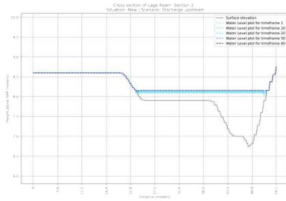
**Figure F.16:** Cross section of the NEW situation of section 2 in the Lage Raam | Scenario: Discharge  $T > 1X25$  year
