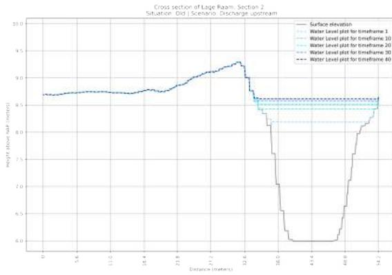
**Figure F.15:** Cross section of the OLD situation of section 2 in the Lage Raam | Scenario: Discharge  $T > 1X25$  year
