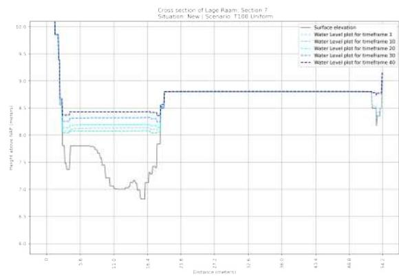
**Figure F.96:** Cross section of the NEW situation of section 7 in the Lage Raam | Scenario: T=1x100 year Uniform Rainfall event
