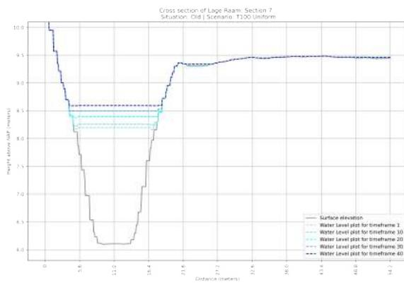
**Figure F.95:** Cross section of the OLD situation of section 7 in the Lage Raam | Scenario: T=1x100 year Uniform Rainfall event
