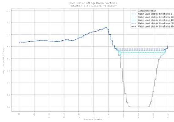
**Figure F.21:** Cross section of the OLD situation of section 2 in the Lage Raam | Scenario: T=1x1 year Uniform Rainfall event
