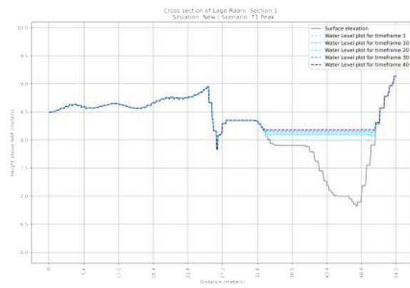
**Figure F.6:** Cross section of the NEW situation of section 1 in the Lage Raam | Scenario:  $T=1x1$  year Peak Rainfall event
