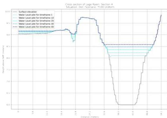
**Figure F.47:** Cross section of the OLD situation of section 4 in the Lage Raam | Scenario: T=1x100 year Uniform Rainfall event
