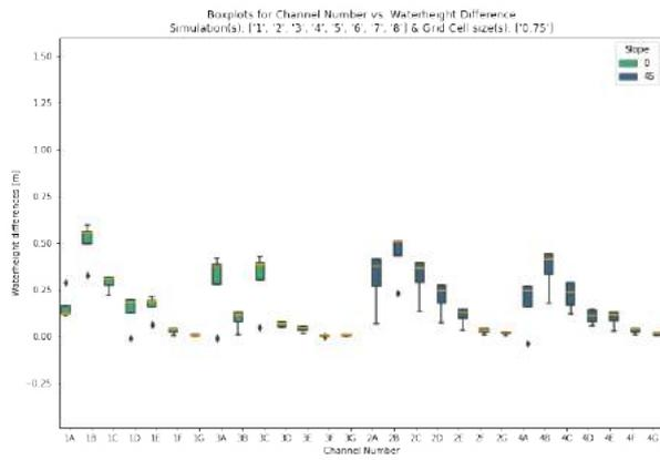
**Figure C.23:** Boxplot for grid placement results divided per channel and angle. Grid cell size: 0.75 meter
