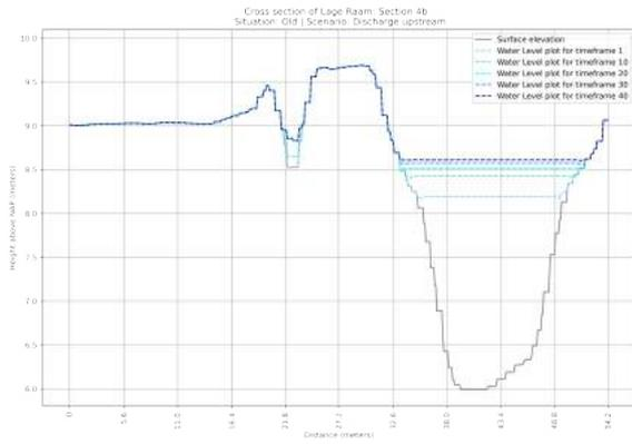
**Figure F.51:** Cross section of the OLD situation of section 4b in the Lage Raam | Scenario: Discharge  $T > 1X25$  year
