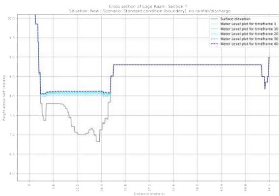
**Figure F.86:** Cross section of the NEW situation of section 7 in the Lage Raam | Scenario: Standard situation
