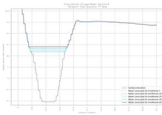
**Figure F.77:** Cross section of the OLD situation of section 6 in the Lage Raam | Scenario:  $T=1x1$  year Peak Rainfall event
