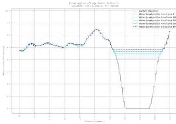
**Figure F.9:** Cross section of the OLD situation of section 1 in the Lage Raam | Scenario: T=1x1 year Uniform Rainfall event
