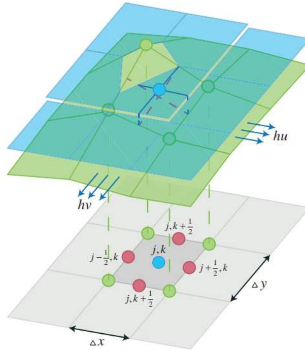
Figure A.6: Visualisation of 2D piecewise linearization on grid (Bollermann et al., 2014)
