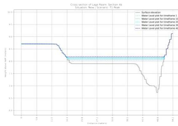
**Figure F.54:** Cross section of the NEW situation of section 4b in the Lage Raam | Scenario:  $T=1x1$  year Peak Rainfall event
