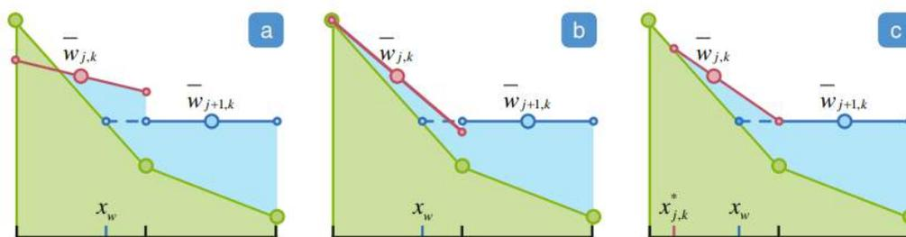
**Figure A.7:** Approximation of the wet/dry front reconstruction. The blue dashed line represents the waterline of the fully flooded cell. (a) Wrong approximation by the piecewise linear reconstruction, which produces a negative value. (b) Positivity preserving but unbalanced piecewise linear reconstruction. (c) Positivity-preserving and well-balanced piecewise linear reconstruction (Bollermann et al., 2014)
