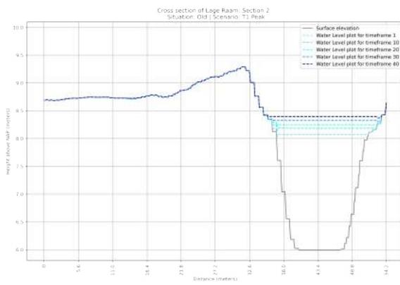
**Figure F.17:** Cross section of the OLD situation of section 2 in the Lage Raam | Scenario:  $T=1x1$  year Peak Rainfall event
