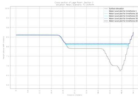
**Figure F.22:** Cross section of the NEW situation of section 2 in the Lage Raam | Scenario: T=1x1 year Uniform Rainfall event
