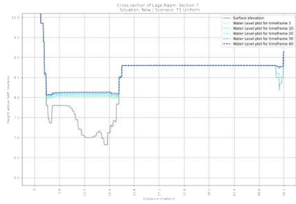
**Figure F.94:** Cross section of the NEW situation of section 7 in the Lage Raam | Scenario: T=1x1 year Uniform Rainfall event
