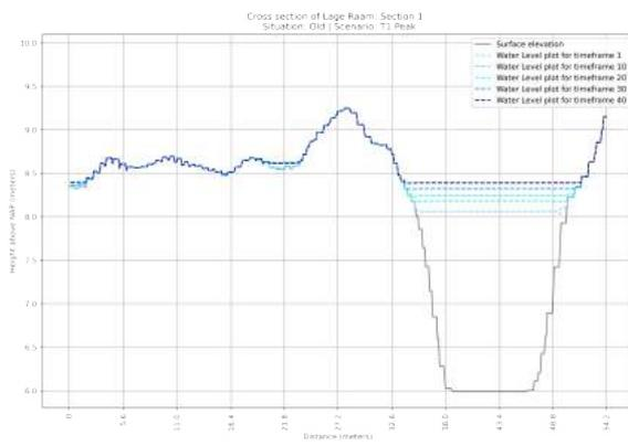
**Figure F.5:** Cross section of the OLD situation of section 1 in the Lage Raam | Scenario:  $T=1x1$  year Peak Rainfall event
