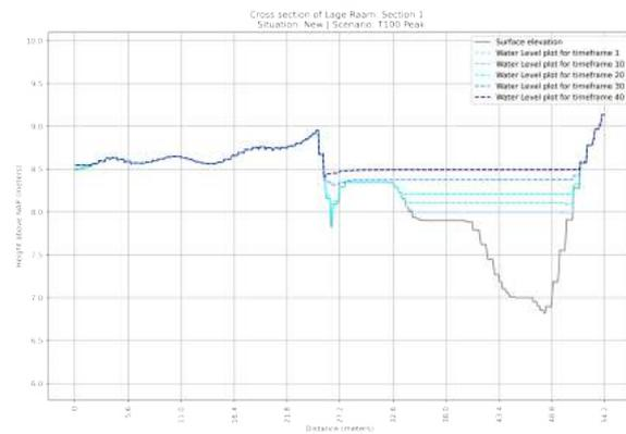
**Figure F.8:** Cross section of the NEW situation of section 1 in the Lage Raam | Scenario:  $T=1x100$  year Peak Rainfall event
