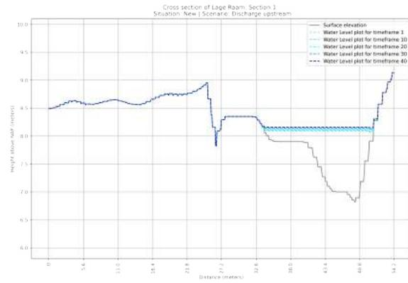
**Figure F.4:** Cross section of the NEW situation of section 1 in the Lage Raam | Scenario: Discharge  $T > 1X25$  year
