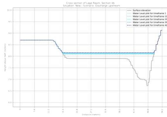
**Figure F.52:** Cross section of the NEW situation of section 4b in the Lage Raam | Scenario: Discharge  $T > 1X25$  year
