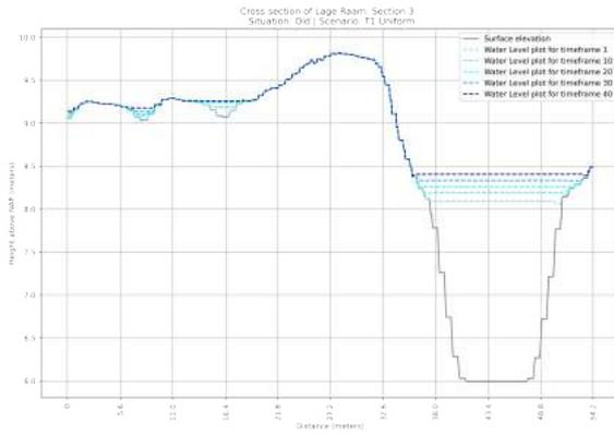
**Figure F.33:** Cross section of the OLD situation of section 3 in the Lage Raam | Scenario: T=1x1 year Uniform Rainfall event
