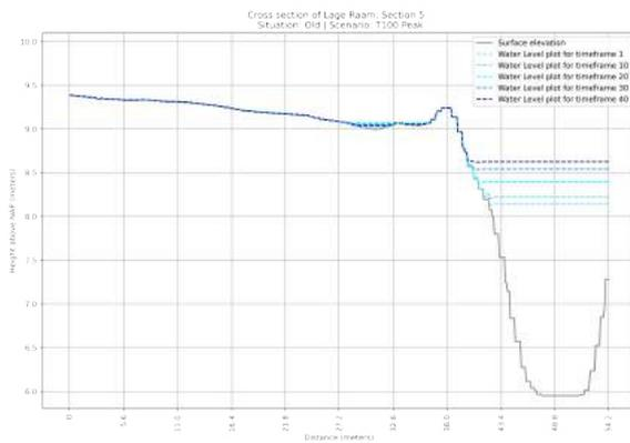
**Figure F.67:** Cross section of the OLD situation of section 5 in the Lage Raam | Scenario:  $T=1x100$  year Peak Rainfall event
