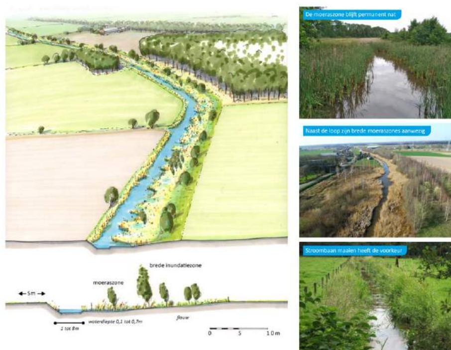
**Figure 7.5:** Target Image of the Lage Raam, R20 type stream with woven nature-friendly banks
