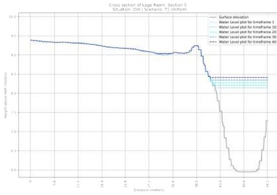
**Figure F.69:** Cross section of the OLD situation of section 5 in the Lage Raam | Scenario: T=1x1 year Uniform Rainfall event
