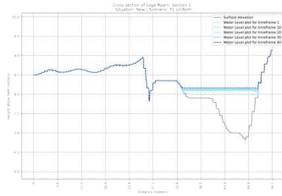
**Figure F.10:** Cross section of the NEW situation of section 1 in the Lage Raam | Scenario: T=1x1 year Uniform Rainfall event
