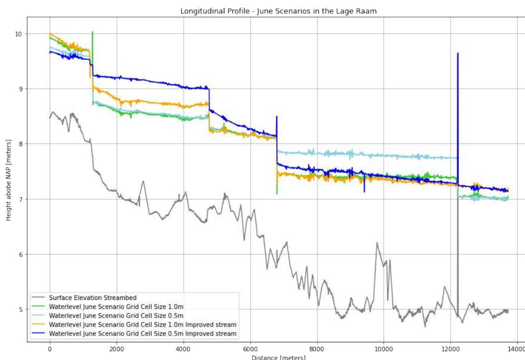
**Figure 10.2:** Example of a waterway incorrectly implemented by open data in Tygron causing bad drainage
