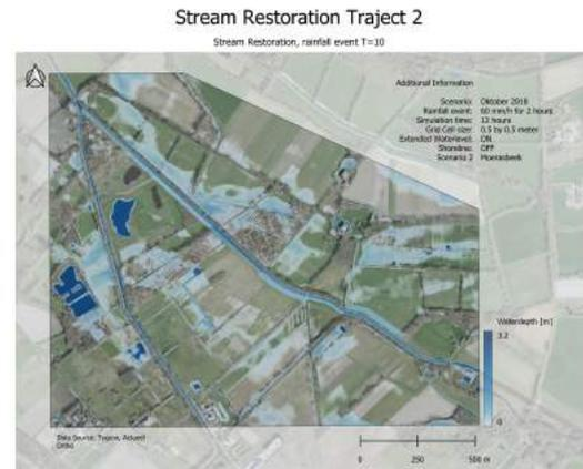
Figure 10.12: Lage Raam case: Scenario 3 with stream restoration profiles
