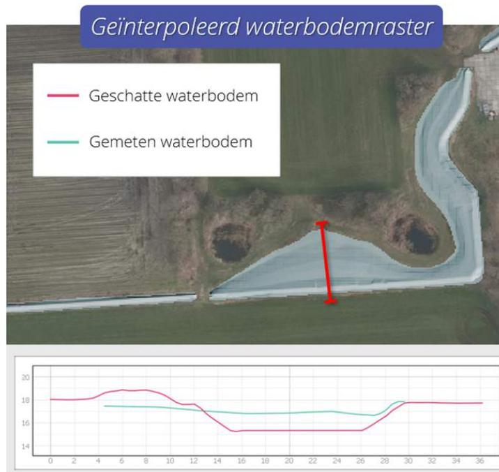
**Figure A.9:** Cross-sections automated in Tygron made of open data vs. cross-sections based on measured profiles in the the Raamvallei
