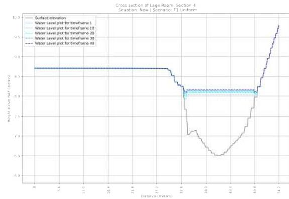
**Figure F.46:** Cross section of the NEW situation of section 4 in the Lage Raam | Scenario: T=1x1 year Uniform Rainfall event
