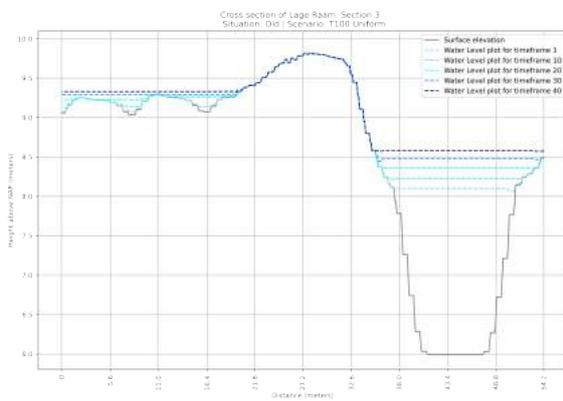
**Figure F.35:** Cross section of the OLD situation of section 3 in the Lage Raam | Scenario: T=1x100 year Uniform Rainfall event
