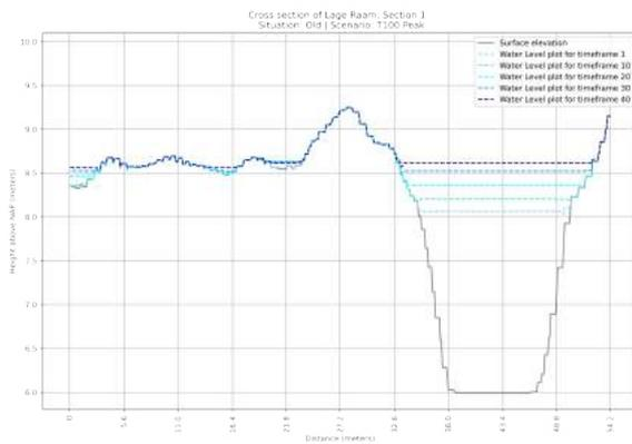
**Figure F.7:** Cross section of the OLD situation of section 1 in the Lage Raam | Scenario:  $T=1x100$  year Peak Rainfall event
