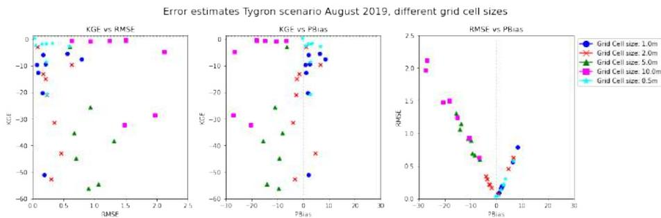
Figure E.6: Estimate error for August 2019 scenario together after validation of the model, each simulation run with different grid cell sizes (gr)
