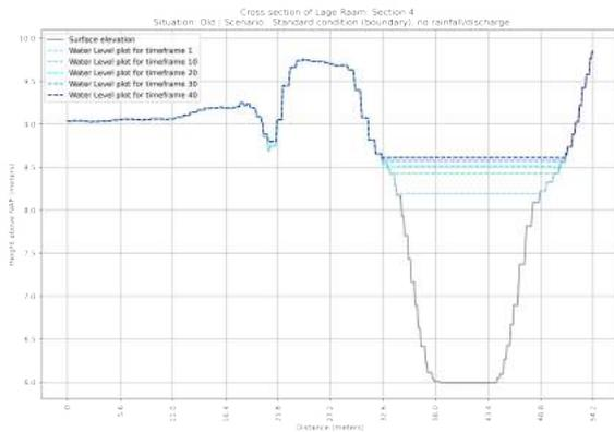
**Figure F.37:** Cross section of the OLD situation of section 4 in the Lage Raam | Scenario: Standard situation
