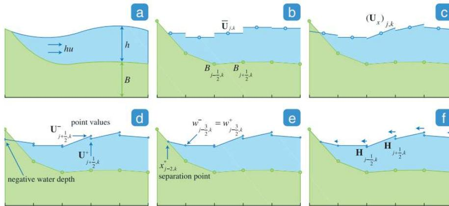
**Figure A.8:** Schematic overview: (f) Fluxes are computed using the central-upwind function at each cell interface (Bollermann et al., 2014)
