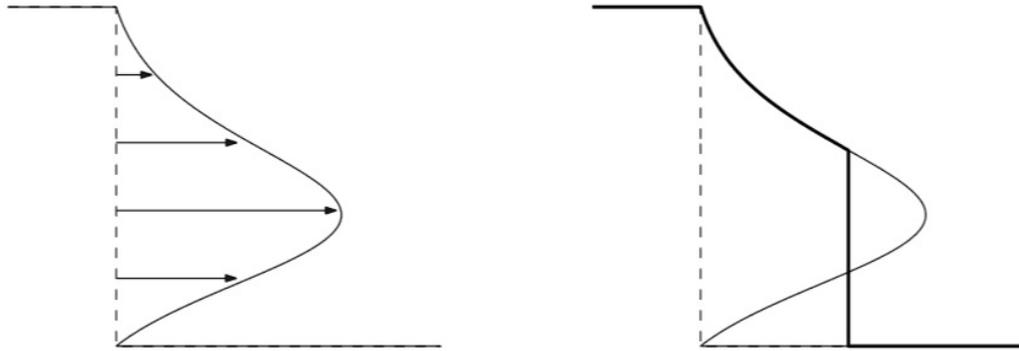
Figure 5.2: Water saturation profile for the Buckley-Leverett solution of a water injection. The correct solution is built from the triple-valued solution by setting the shock wave at the front of the advancing water.
