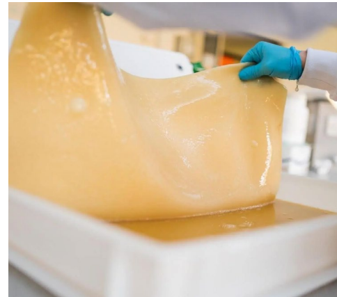
Figure 37: laboratory inoculation and culture preparation, controlled BC growth, pellicle harvesting and shaping into functional material forms. Source: Nexio Projects (n.d.), BMS (n.d.), University of Exeter (n.d.), Foamlab (2025).
