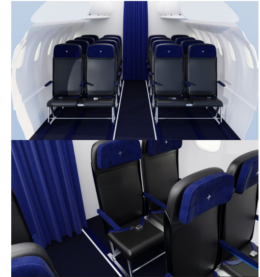
Design B (New CMF Design from this thesis in a wide angle view and close up view render)
