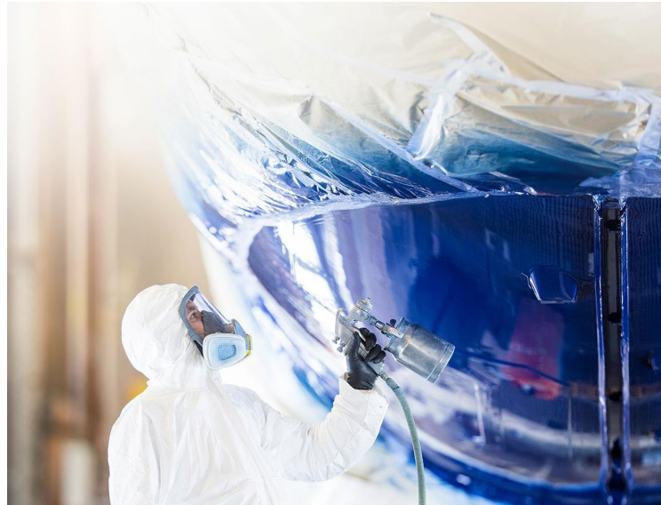
Usage of water-based primers, paints and adhesives, reducing VOCs by over 75% (Embraer sustainability report, 2024)
