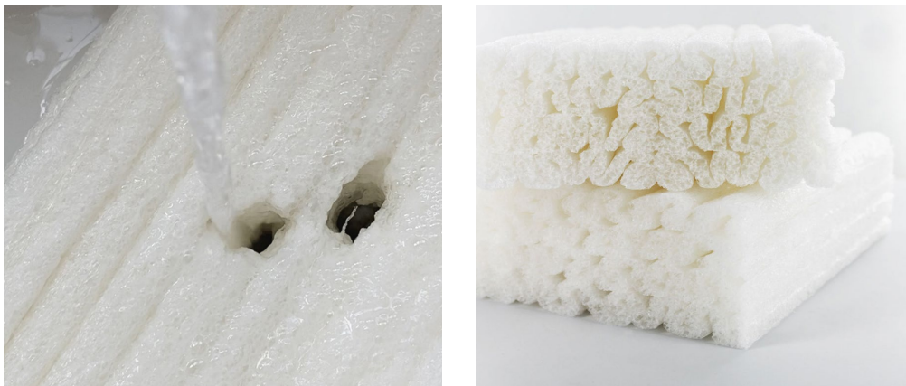
Figure 29: Zouch Converters water dissolvable biodegradable foam packaging. Source: Zouch Converters Ltd. (n.d.).
