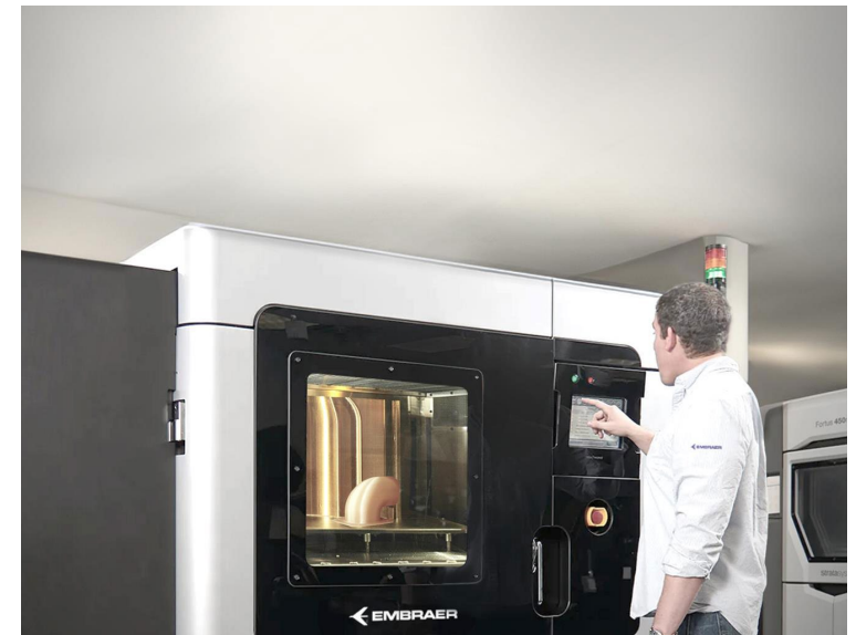
Building the aircraft with 3D printers (over 60% of the cabin parts, cutting weight by 40% and waste by 65%). (Embraer additive manufacturing, 2023)
