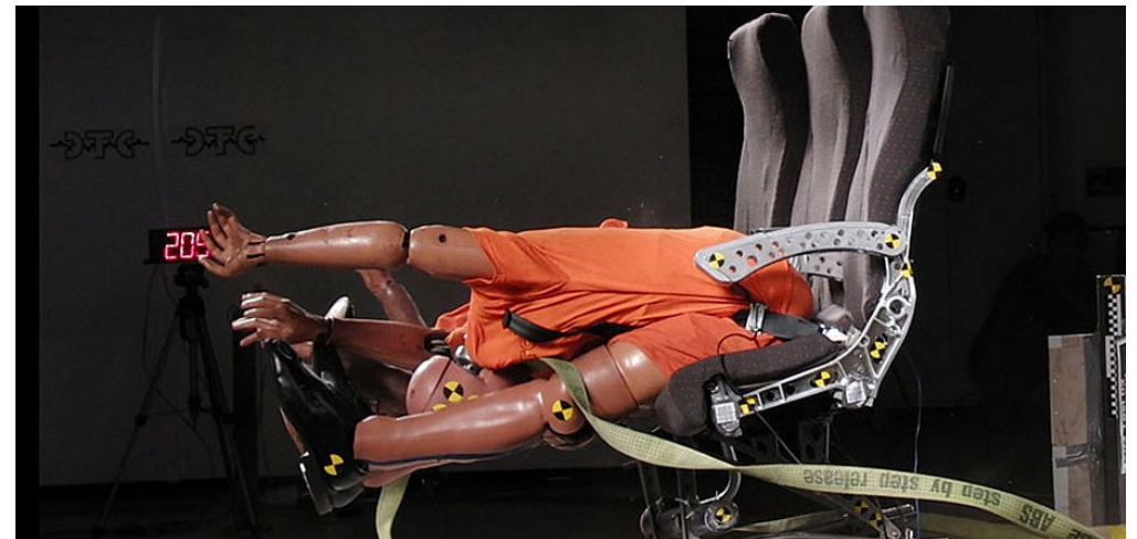
Figure 20: Dynamic 16G forward crashworthiness test of aircraft seats. Source: Federal Aviation Administration (FAA) (n.d.).
