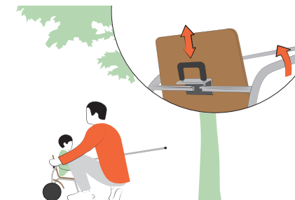
Figure 5.6: Opening the cart. The pull bar can be rotated upwards after pulling the handle .
