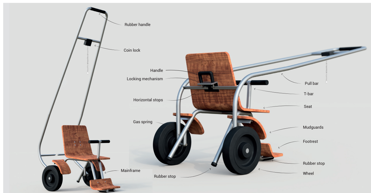
Figure 6.10: Two renders of the cart in open and closed position, arrows point at main elements
