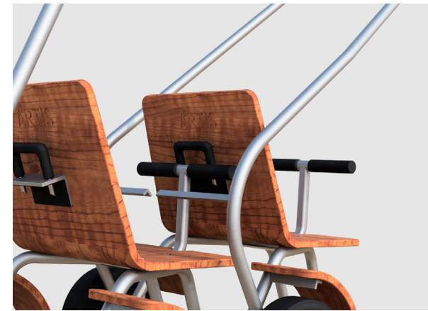
Figure 6.14: Render of two carts, pull bar sliding along T-bar of the cart behind when rotating pull bar upwards.
