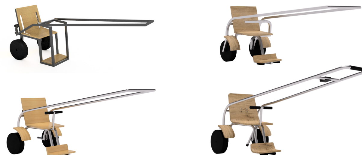
Figure 4.9: Images from top left (first) to bottom right (final) show progress of the concept using 3D models
