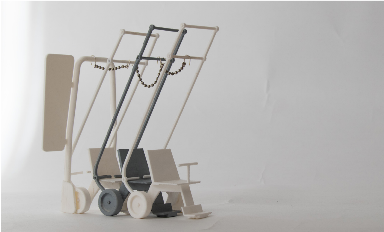
Figure 6.7: Scale model (1:10) of carts in docking station, showing main frame and information sign
