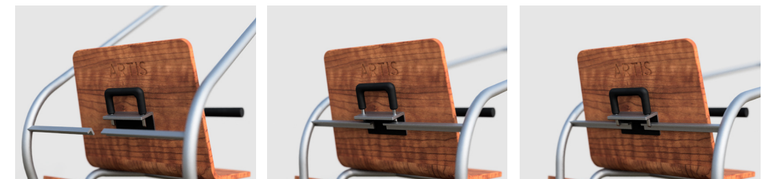
Figure 6.12: Movement of indexing pins, pull bar approaching the lock, indexing pins moving upwards, indexing pins automatically lock the horizontal stops
