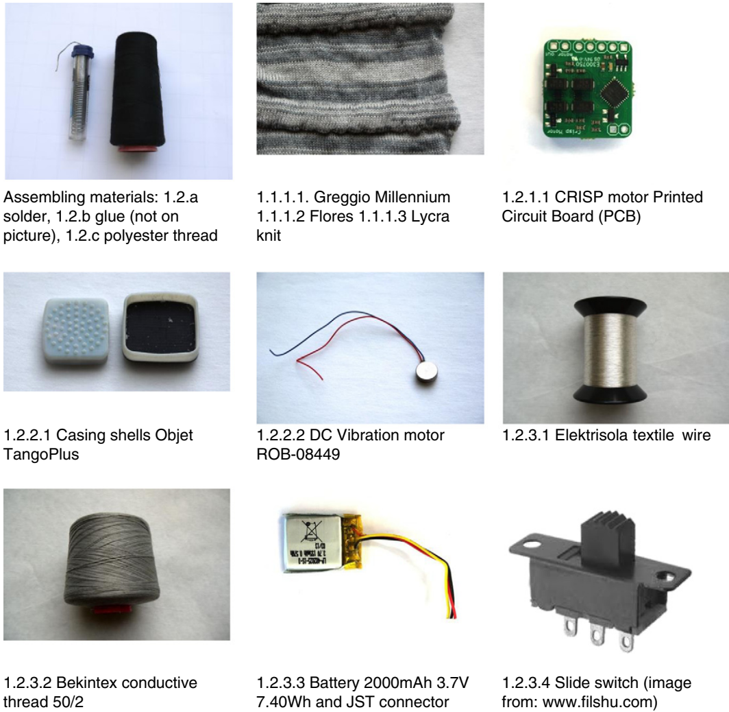
Fig. 7. Photos of the textile and electronic materials used in Vibe-ing.
