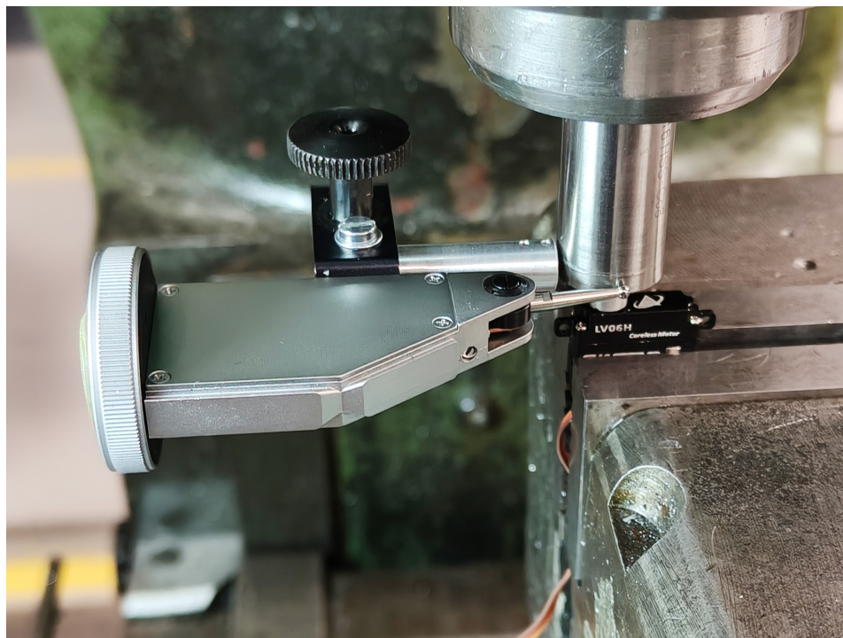
Figure 4.4: Locating the center of rotation of the servo
