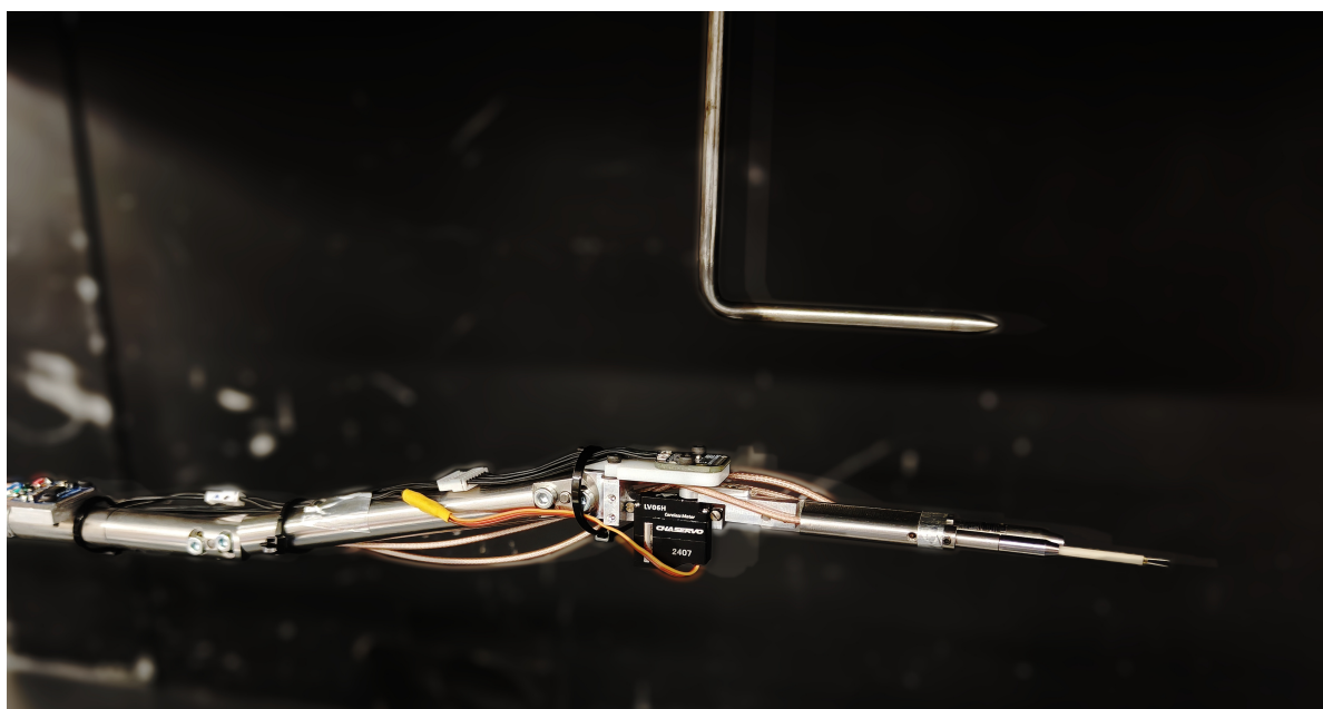
Figure 4.12: Calibrator and pitot tube in the M-tunnel of the LSL
