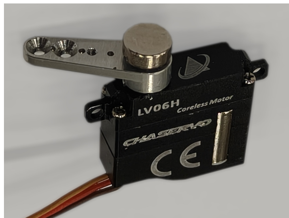
Figure 4.6: Servo with the magnet aligned and adhered
