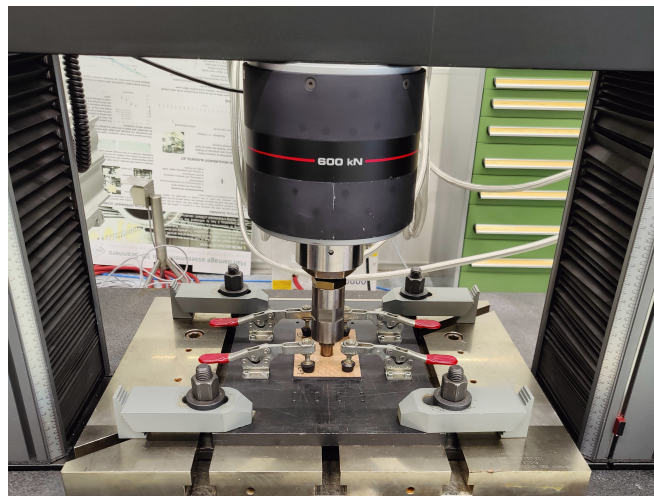
Figure 6.1: A Coupon Sample in the Compression Test Bench
