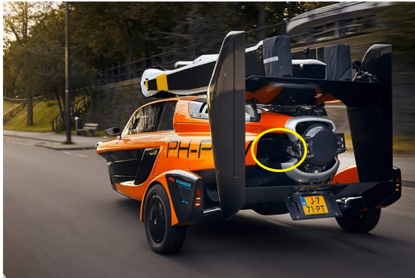
Figure 4.10: A View at the Folded Propeller in Drive Mode with the Exposed Propeller circled in Yellow. image credit: PAL-V
