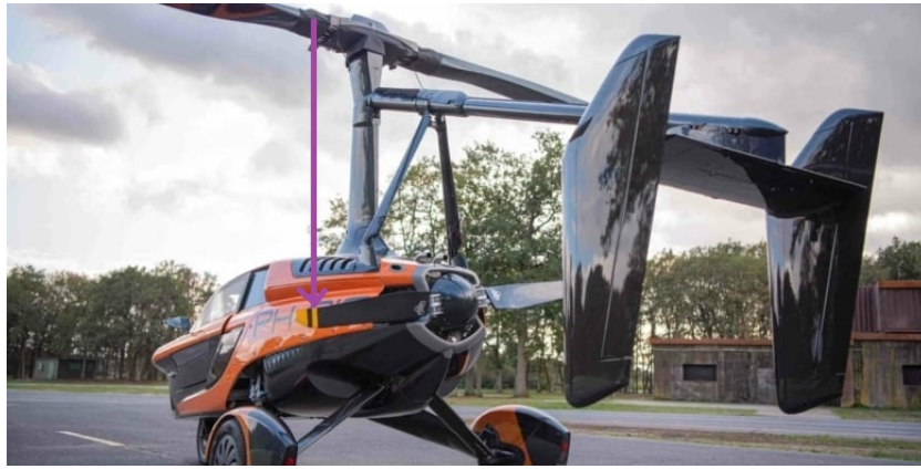
Figure 4.12: Rear View of the PAL-V Liberty in Fly Mode. With a tool drop scenario in purple. image credit: PAL-V
