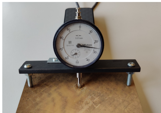
Figure 6.6: The Dial Indicator used for Dent Depth Measurements
