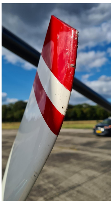
Figure 4.9: FOD Impact on the PAL-V Liberty Test Vehicle. image credit: PAL-V
