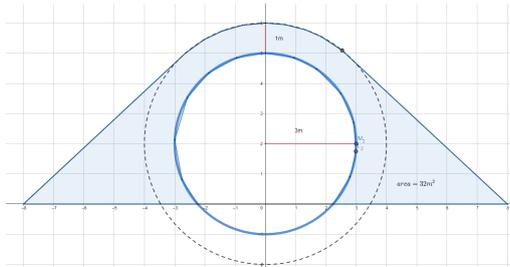
**Figure 7.5:** Cross section drawing of the regolith over the livable section of the habitat. Dotted lines show the minimum amount of regolith required, and the blue area shows where the regolith bags would be
