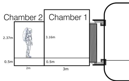
Figure 7.10: Side view of the airlock including the dimensions
