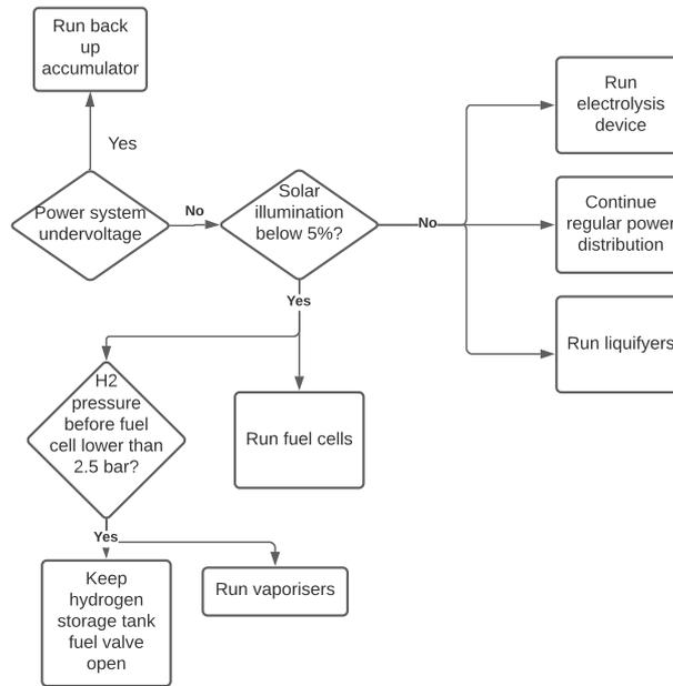
Figure 9.6: Software diagram of the power distribution system
