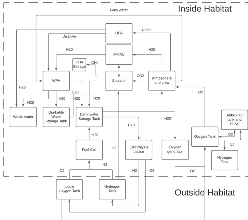
Figure 10.7: Hardware diagram of the life support and power subsystems
