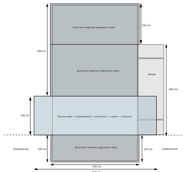
Figure 12.2: Safe house's external layout visualisation of the different protective layers.
