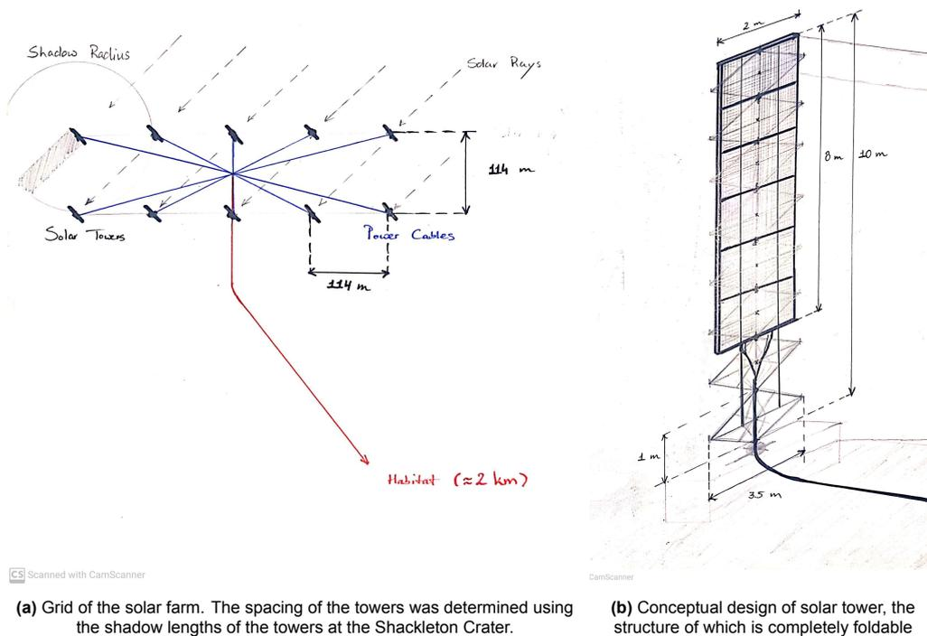
**Figure 9.3:** Solar power generation system infrastructure
