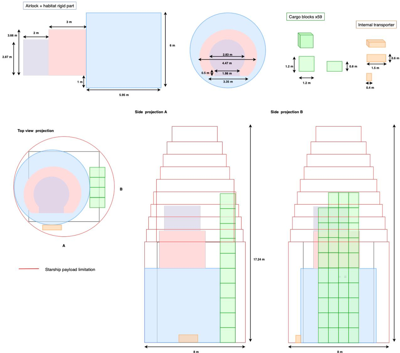
**Figure 13.5:** Starship payload configuration for launch 2
