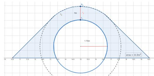
**Figure 7.6:** Cross section drawing of the regolith over the innermost airlock chamber. Dotted lines show the minimum amount of regolith required, and the blue area shows where the regolith bags would be
