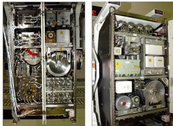
Figure 10.2: The ISS Water Recovery System consisting of WRS 1 on the left and WRS 2 on the right. The Water Processor Assembly is contained in WRS 1 and the right half of WRS 2. The Urine Processor Assembly is in the remaining left half of WRS 2.<sup>1</sup>
