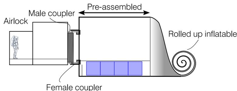
Figure 7.11: Coupling System of the Airlock and the Inflatable Structure
