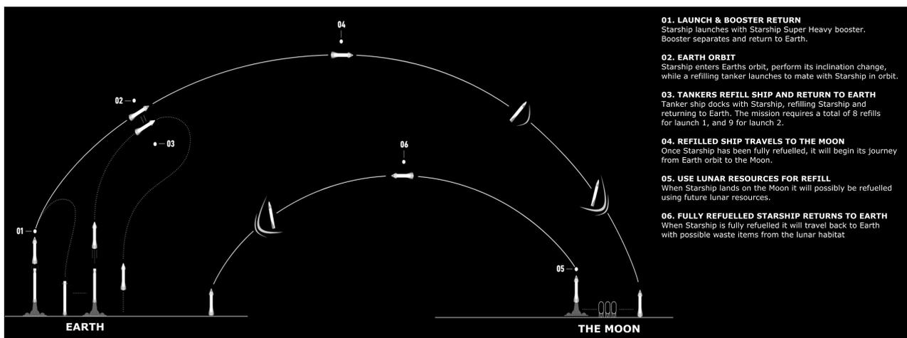
**Figure 13.3:** Travelling from Earth to the Moon using a Starship spacecraft, Super Heavy rocket and tankers
