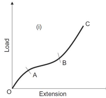
Figure 7.4: Common tensile behaviour of a fabric. Initial region [OA], decrimping region [AB], and yarn extension region [BC] are all exaggerated for visibility
