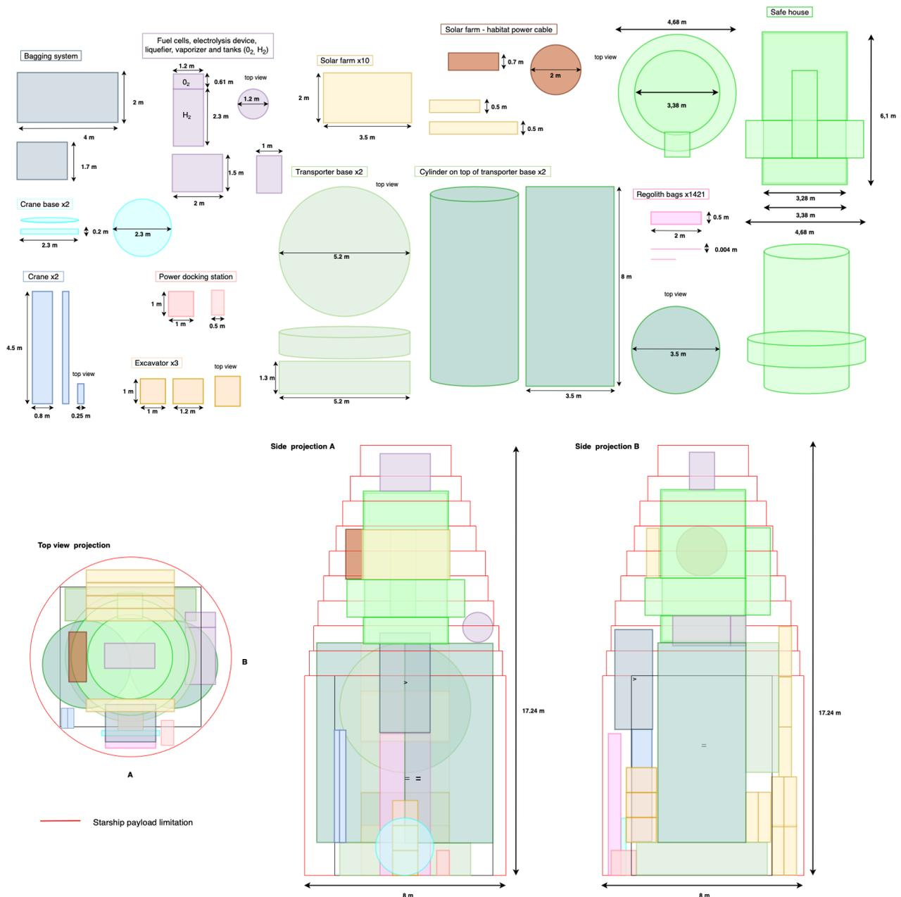
Figure 13.4: Starship payload configuration for launch 1
