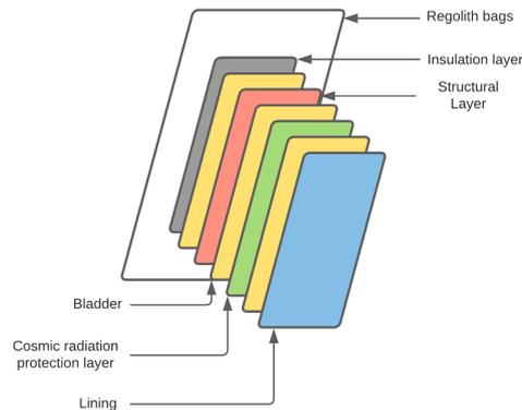
Figure 7.2: Schematic of the different layers of the habitat
