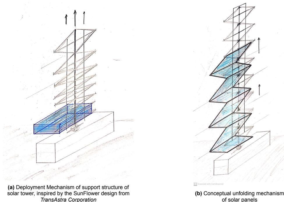
**Figure 9.2:** Solar tower assembly unfolding mechanisms.
