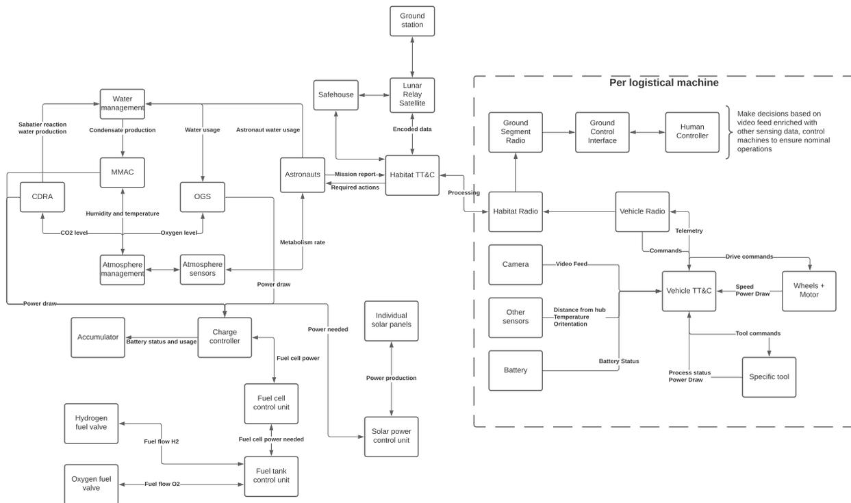
**Figure 14.1:** Communication flow diagram of the various subsystems and the astronauts.
