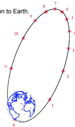
**Figure 14.2:** Schematic drawing of a Molniya orbit around Earth, in which the majority of the orbital period is spent in contact with the ground station. [31]
