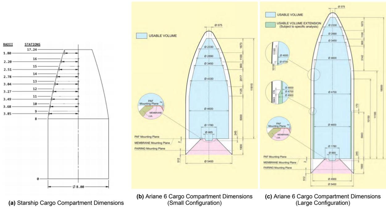
Figure 13.1: Cargo compartment dimensions of both the Starship and Ariane64 [102][3]
