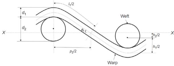
Figure 7.3: Schematic of a plain weave [6]
