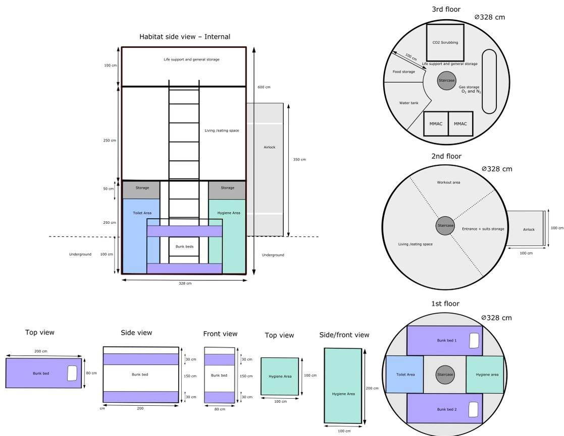
Figure 12.1: Safe house's internal layout of its different floors including dimensions.
