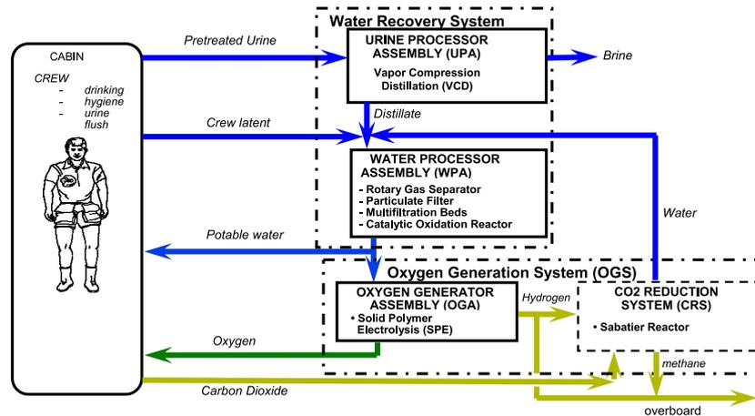
Figure 10.1: Diagram showing the interactions between the subsystems of the Water Recovery and Management System of the US ISS segment. [14]
