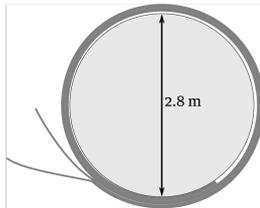
Figure 7.14: Dimension of Rolled Up Inflatable Structure
