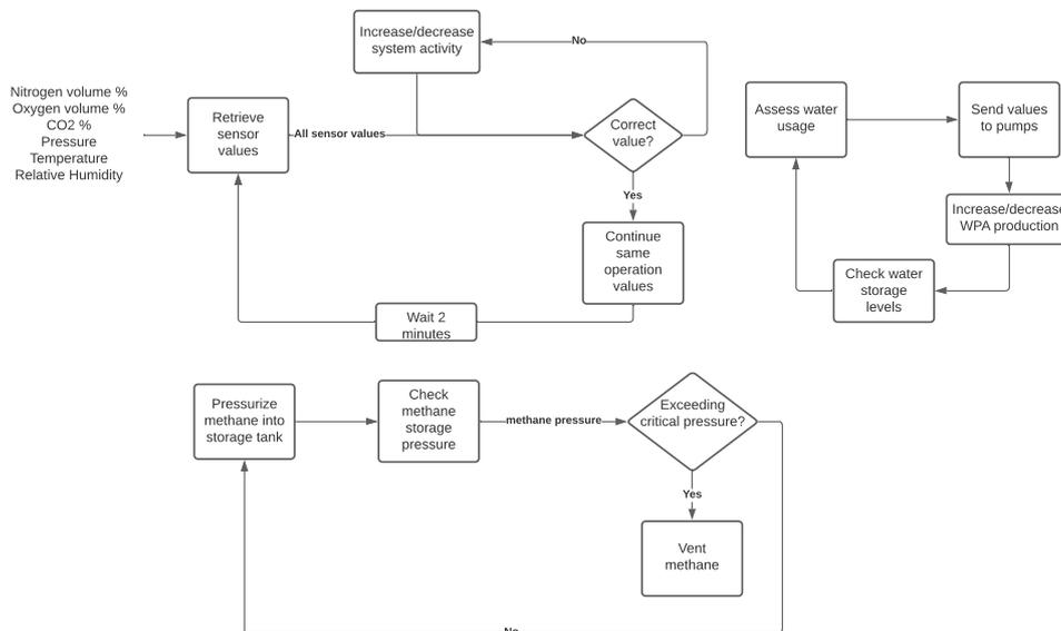
Figure 10.8: Software diagram of various subsystems within life support.
