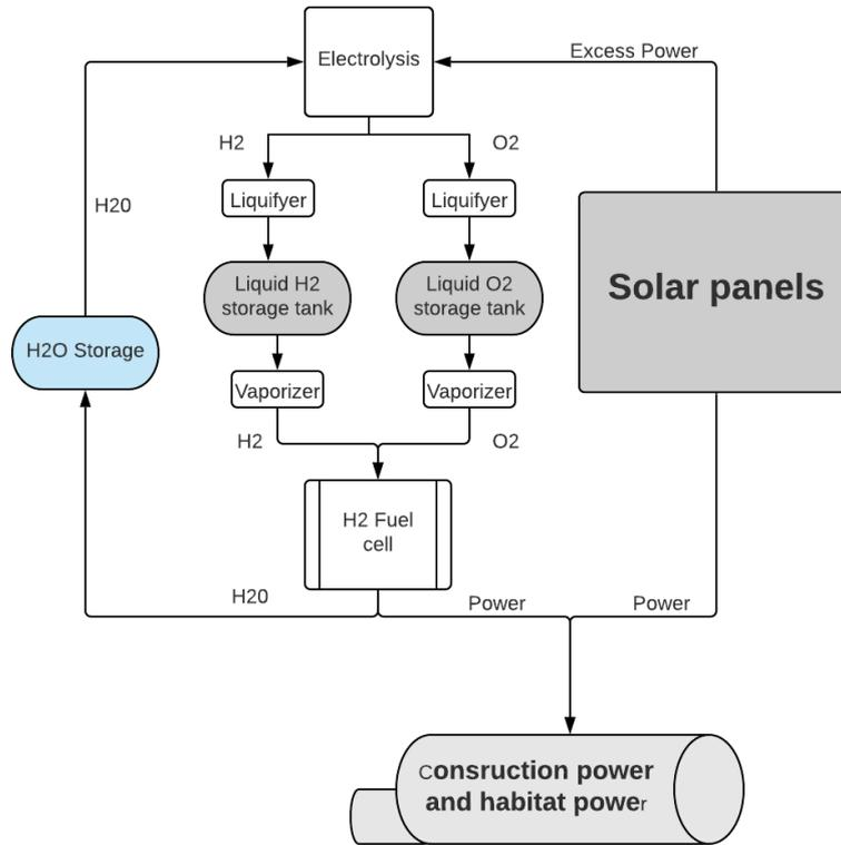
Figure 9.1: Overview of regenerative fuel cell system
