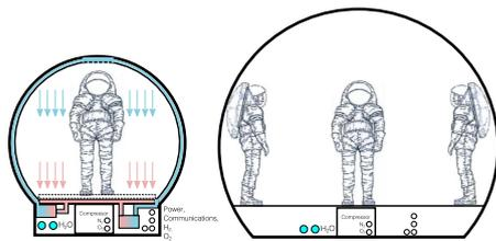
Figure 7.9: Front view of the airlock, showing the necessary equipment and pipes to connect with outside systems.
