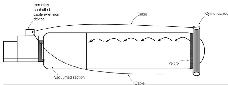
**Figure 8.3:** Unrolled Inflatable Structure
