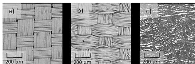
**Figure 7.7:** Comparison of plain woven (a), ripstop woven (b), and non-woven (c) fabrics[21]
