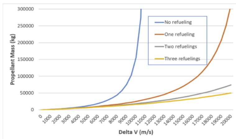
Figure 2.3: The effect of refuelling on the growth of required propellant with growing  $\Delta V$  [100]
