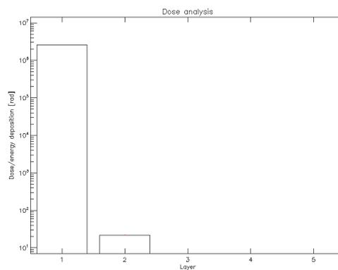
**Figure 4.6:** Simulation for an extreme SPE with SAPPHIRE (1 in 1000 year event) with the layers in configuration 1
