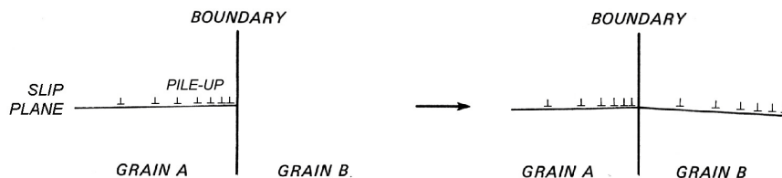
Figure 12.14. Spreading of slip from one grain to another.
