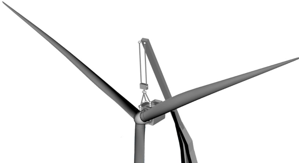
Figure 2.5: Rigging arrangement for installing the RNA using three slings from crane block to lift frame. The lift frame is rigidly connected to the RNA. The nacelle is modelled as one body and the rotor as another body that is rigidly connected to the nacelle
