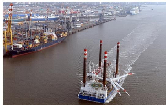
Figure 1.4: Victoria Matthias from MPI Offshore (jack-up vessel) with pre-assembled rotors on the main deck (Eurogate).
