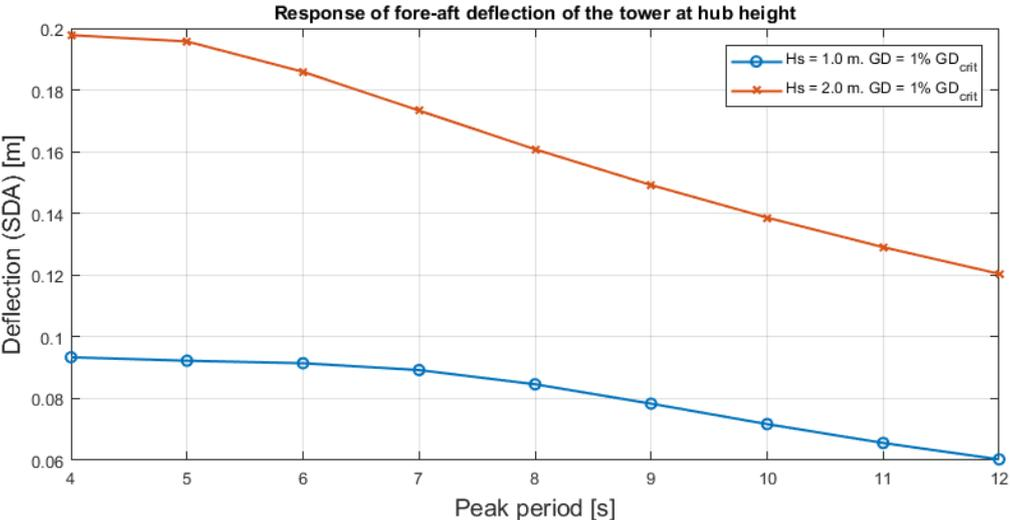
Figure 3.8: Significant response as SDA of the fore-aft deflection of the tower at hub height for different  $T_p$ ,  $H_s = 1.0$  and  $2.0$  m and damping as 1% of the critical damping of the structure.
