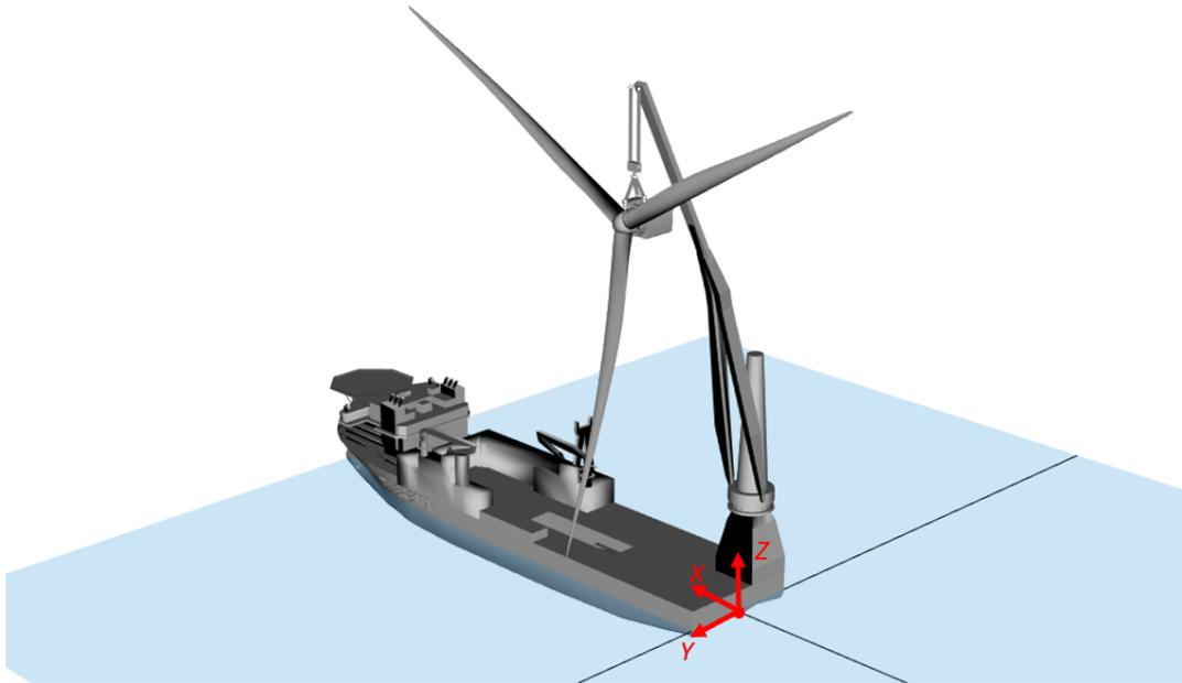
Figure 7.1: Overview of *Model 3 - Wind & Waves*. The global coordinate system is shown as well, which has its origin at MSL, stern, centerline of the vessel.
