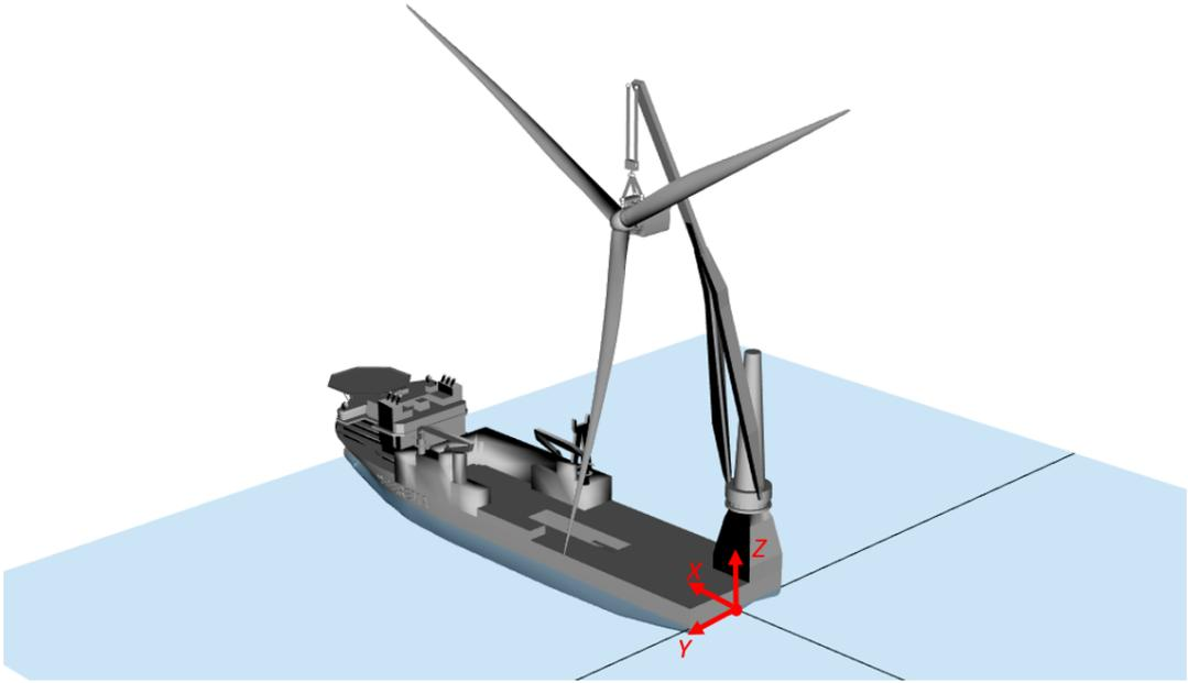
Figure 6.1: Overview of *Model 3 - Wind & Waves*. The global coordinate system is shown as well, which has its origin at MSL, stern, centerline of the vessel.
