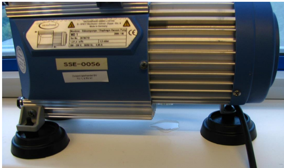
Figure 124: Water Condensation inside the Vacuum Pump
