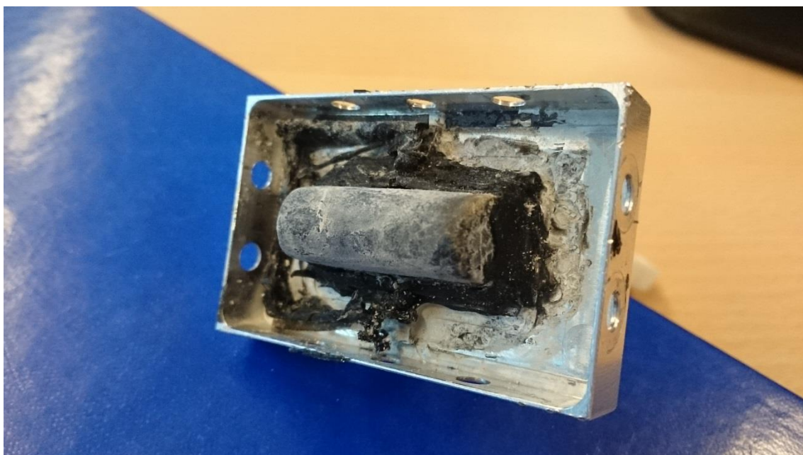
Figure 128: Post Testing Heater Inspection
