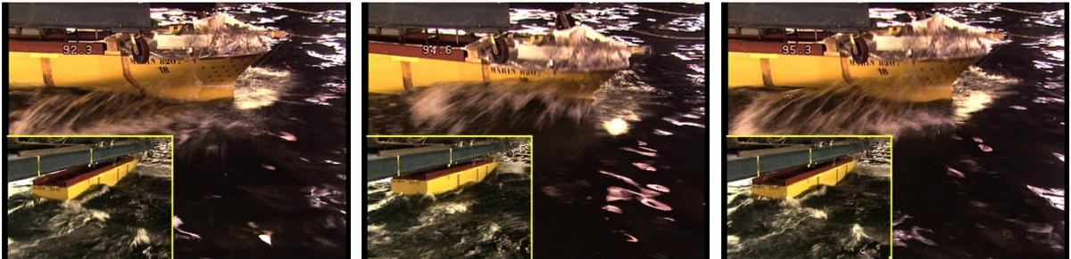
*Figure 8.23: Stills from the video of the forced pitch oscillations, bow quartering waves, heading 150 deg,  $v_S = 20$  kt. The phasing of the forced motion and the incoming regular wave is such that it results in a maximum force on the bow segment.*
