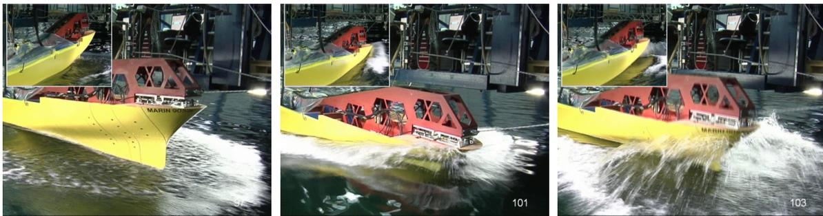
Figure 8.10: Stills from the video of the experiments, the start of the impact at  $t = 101$  s, the maximum immersion of the model and the moment the spray drops back in the water.
