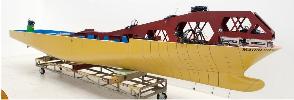
Figure 4.7: Model of the ferry with 10 segments in the forward part of the hull
