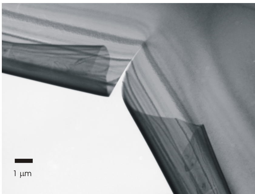
Fig. 2.4. Bending and curling of a MgO foil due to stresses induced by 100 keV Au ion irradiation.
