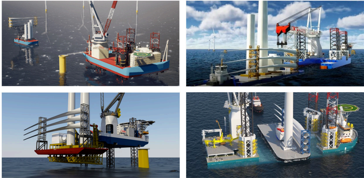
Figure G.1: Feeder concepts clockwise from top left: Maersk concept [112], Feederdock concept [113], Havfram concept [114] and Bargerack concept [115]
