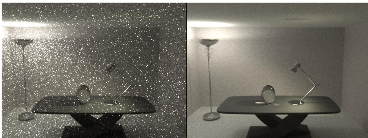
Figure 2.4: Comparison of noise using straightforward path tracing and bidirectional path tracing with the same time limit. The quality improvement is a result of more effective sampling.
