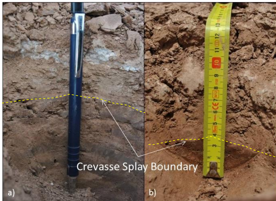
Figure 10. Boundary definition using Color as indicator. a) Crevasse Splay 1 point 25. b) Crevasse Splay 2 point 8.
