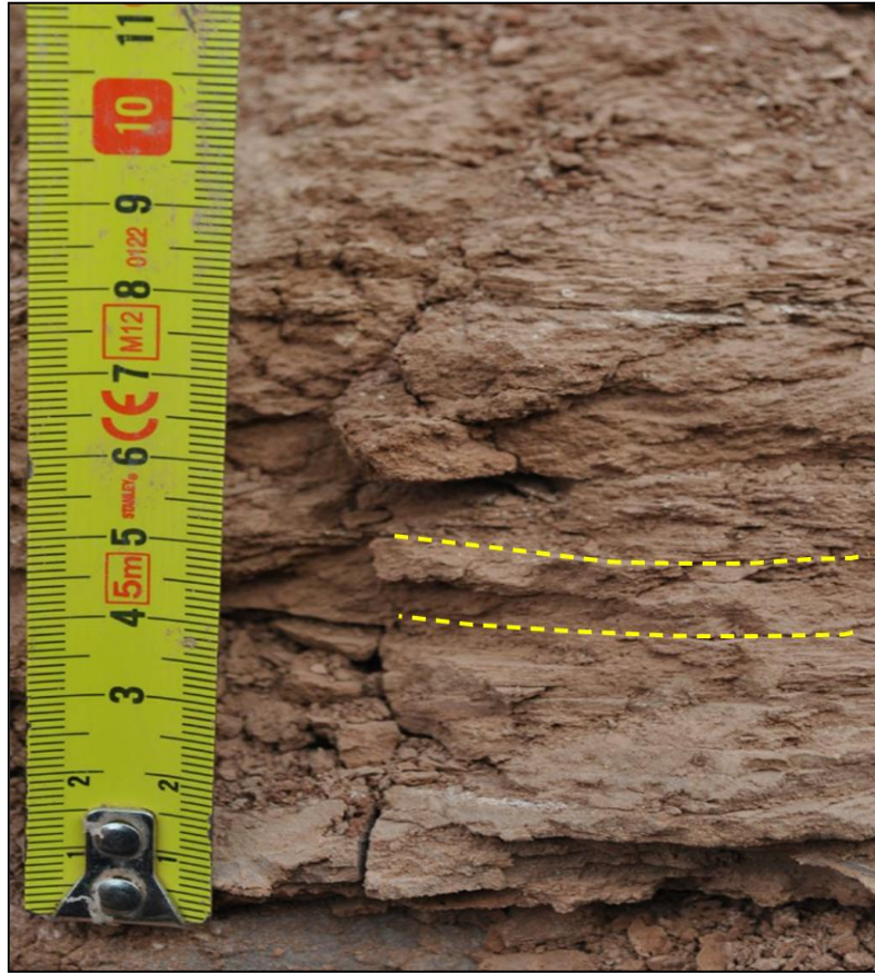
Figure 23. Wavy and Horizontal laminae Silt facies. Crevasse Splay 2
