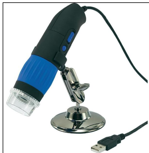
Figure 11. Conrad DP-M17 USB Digital Microscope, 10x to 200x Magnification, 9.0 Megapixel High Resolution.
