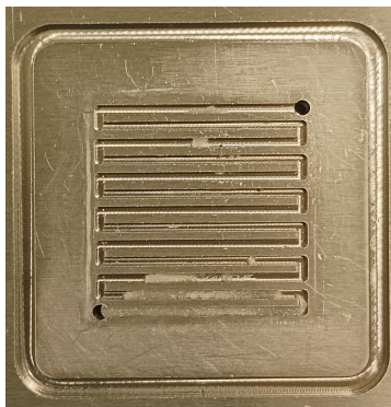
Figure 4.17: Heavy salt precipitation in the bottom rows of the cathode flow channel in the experiment with 0.5 M \text{CsHCO}_3 .
