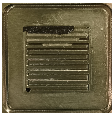
Figure A.5: Heavy salt precipitation in the upper rows of the cathode flow channel in the experiment with 2 Nm bolt compression with the CO_2 gas fed from the bottom nozzle.
