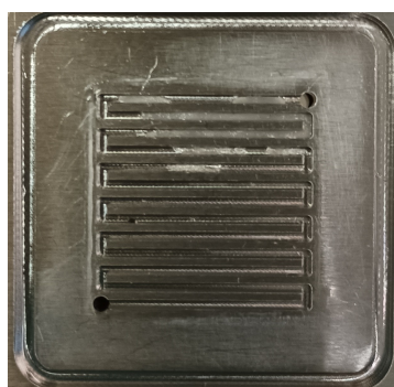
Figure 4.12: Heavy salt precipitation in the upper rows of the cathode flow channel in the experiment with 2 Nm bolt compression.
