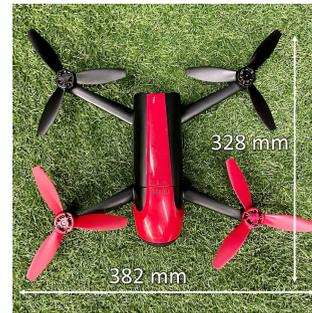
FIGURE 23. Top view of a Parrot Bebop 2 drone.
