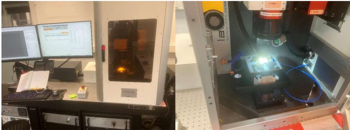
Figure 66: Lasea laser cutter.
