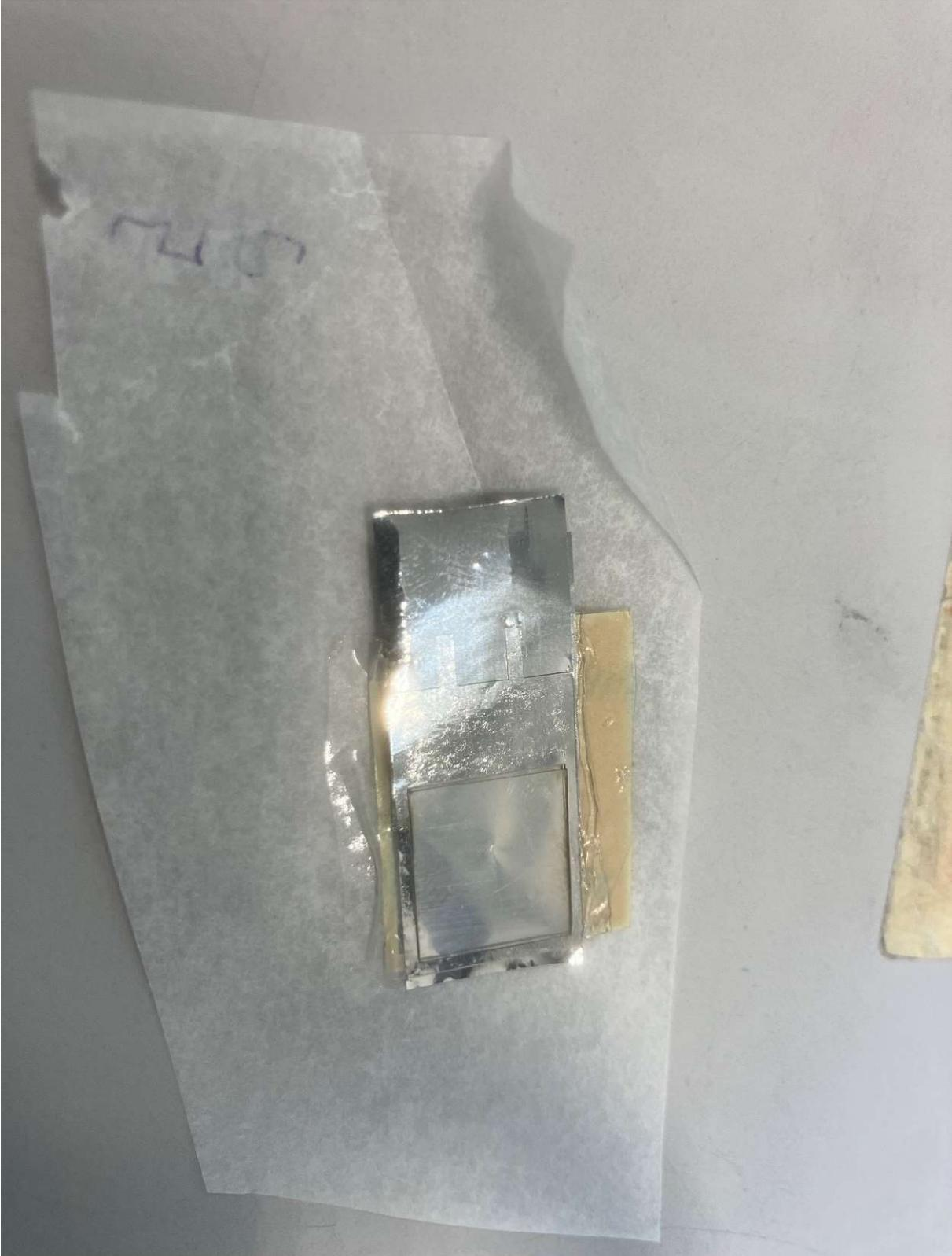
Figure 68: Adhesion layer on top of steel strip, with PVDF film placed in the corresponding hole.
