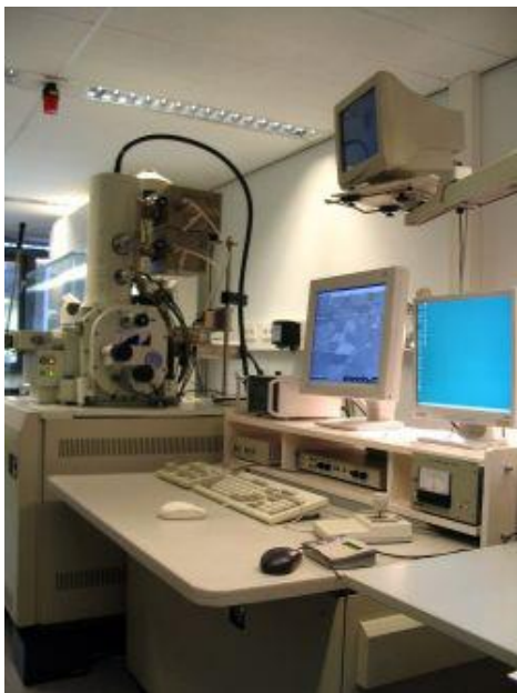
Fig. 2.2: SEM set-up used for examination of PEO layers, at 3ME faculty from TU Delft.
