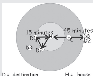
Illustration 14.19: The principle of time-space activity zones. The number of activities that can be carried out by an individual in the course of a single day increases along with the degree to which their 'carriers' are located in one another's vicinity, or on the route from one to another. With a maximum amount of available travel time of 90 minutes per day, point D3 is inaccessible if criss-cross trips are called for
