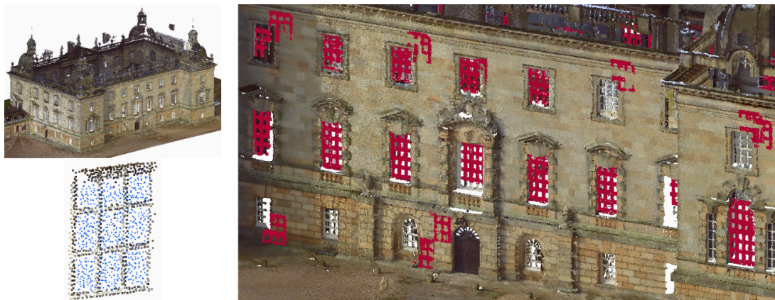
Figure 4.26 – Window detection (red) in the HH dataset using the orientation-aware hit-or-miss transform, blue represents the negative SE
