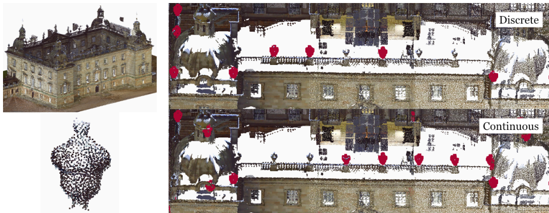
Figure 4.27 – Acorn detection on the HH facade (red) using the density-aware opening: discrete (top) and continuous (bottom)
