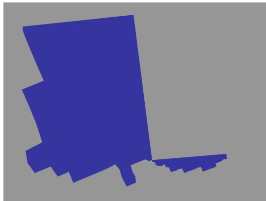
Figure 3.12.: faceAgglomerate output for one of its agglomerations. This non-manifold face is going to fail in the viewFactorsGen step.
