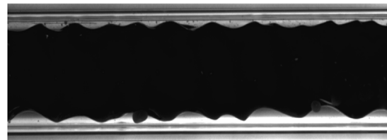
Fig. 7. Flow visualisation of core-annular flow for an oil flow rate of 0.35 l/s and a watercut of 20%. Left: oil viscosity of 2500 cSt ( T_{oil} \approx 23.4^\circ\text{C} ). Right: Oil viscosity of 768 cSt ( T_{oil} \approx 39.0^\circ\text{C} ).
