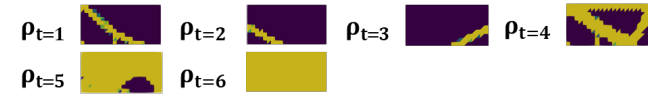
(c) Unfiltered topologies for 6 templates per type resulting in a compliance value of the design of 3.5765 \times 10^{-4} J.
