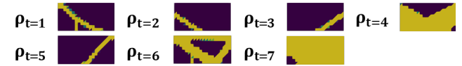
(b) Unfiltered topologies for 7 templates per type resulting in a compliance value of the design of 3.4830 \times 10^{-4} J.
