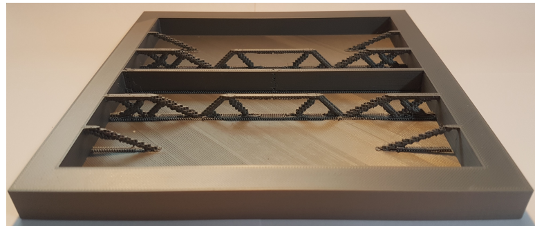
(a) Image of the 3D printed result of the simply stiffened plate for the case of 3 templates per type. The shown result deviates from the one presented in the paper, for this result the upper value of the volume constraint was set to V_{\max} = 0.33 \cdot V_{\text{init.stiff.}} .
