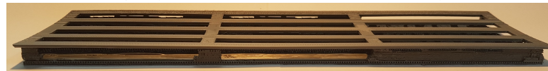
(c) Image of the 3D printed result of the orthogonally stiffened fuselage shell for the case of 3 templates per type.
