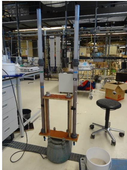
Figure 3-6 The columns with extensions placed on the shaker during filling.
