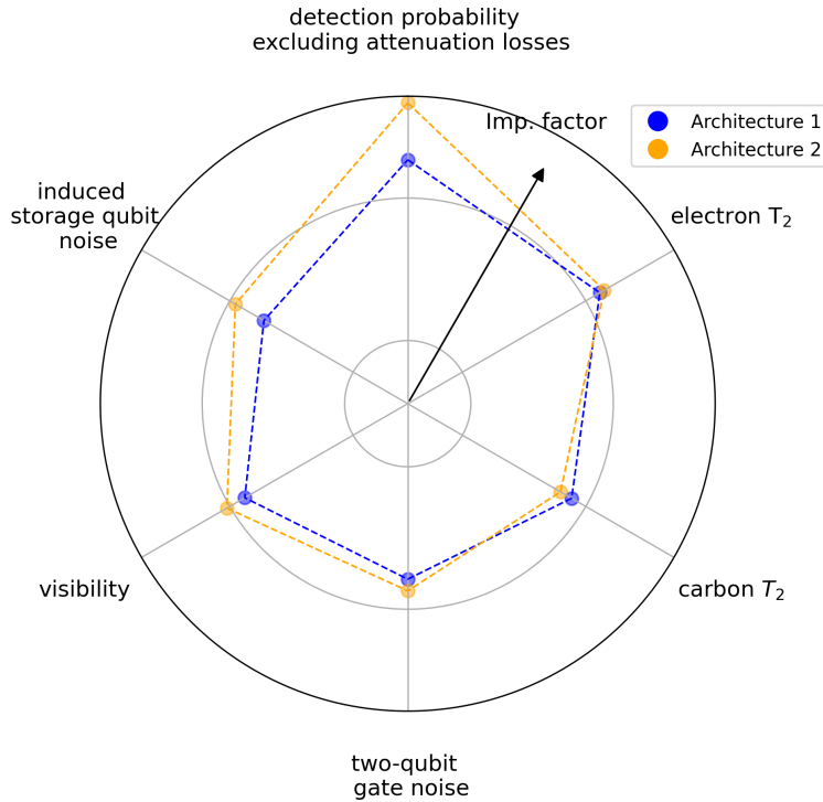
Figure 3.18: Directions along which color-center hardware must be improved to achieve entanglement generation rate R = 0.1 Hz and teleportation fidelity F_T = 0.8717 , enabling VBQC between Delft and Eindhoven, assuming that a double-click entanglement generation protocol is used. The blue (orange) line corresponds to the direction of hardware improvement for the architecture shown on the left (right) in Figure 3.7. Note the use of a logarithmic scale.
