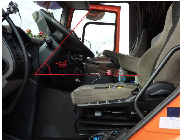
b) Steering wheel inclination angle of a Truck Steering System
