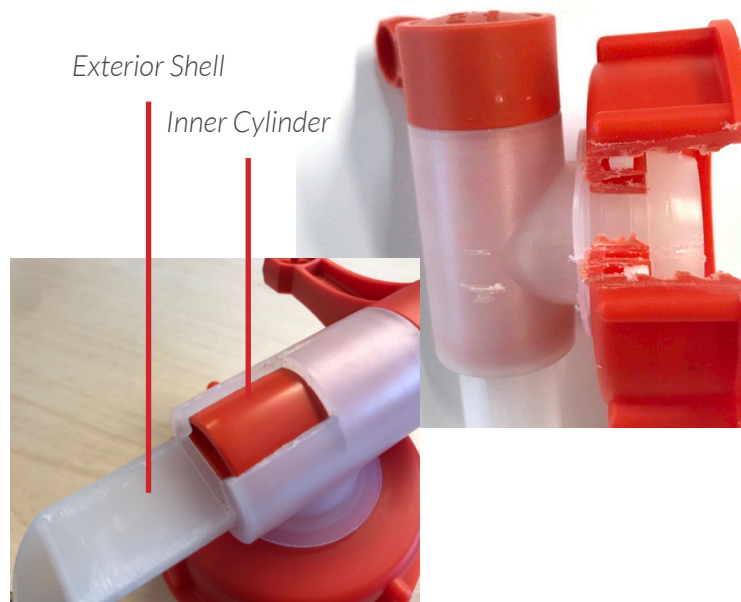
Figure 55: A stiffer and, slightly larger inner cylinder compresses against the exterior shell, creating a waterproof seal.
