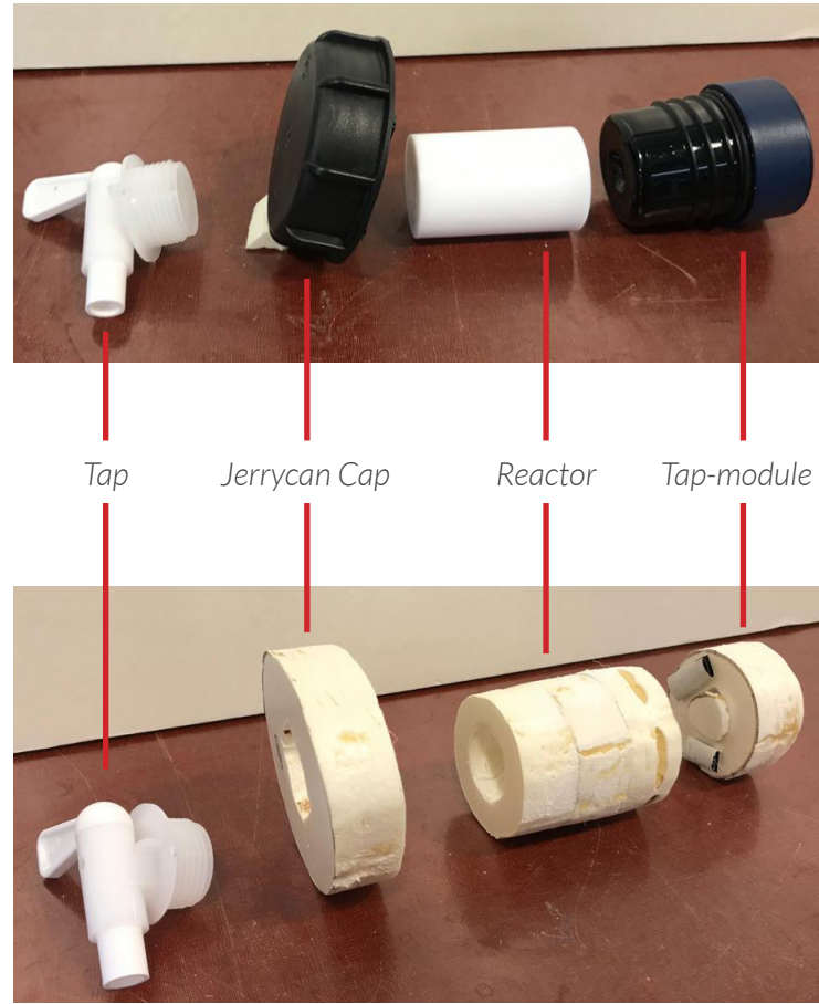
Figure 54: Crucial components for the "tap" concept, from left to right: tap, cap, reactor and the UV-C module.
