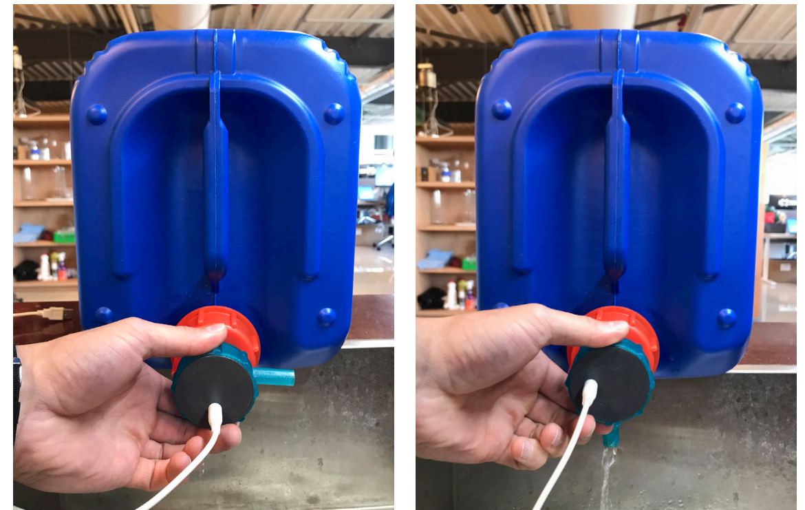
Figure 105: The UV-Tap in use with the charger plugged in. The place of the charger allowed in both on or off position for comfortable use.
