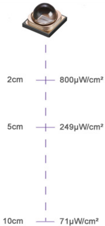
Figure 63: Example of how much the irradiation distance influences the UV-C dose.
