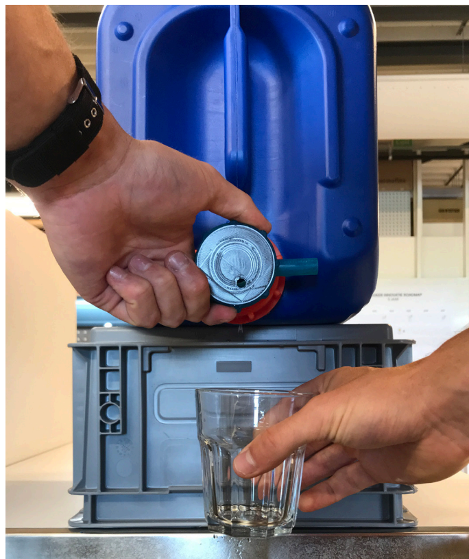
Figure 100: Opening and closing of the UV-Tap demonstrate with a prototype.
