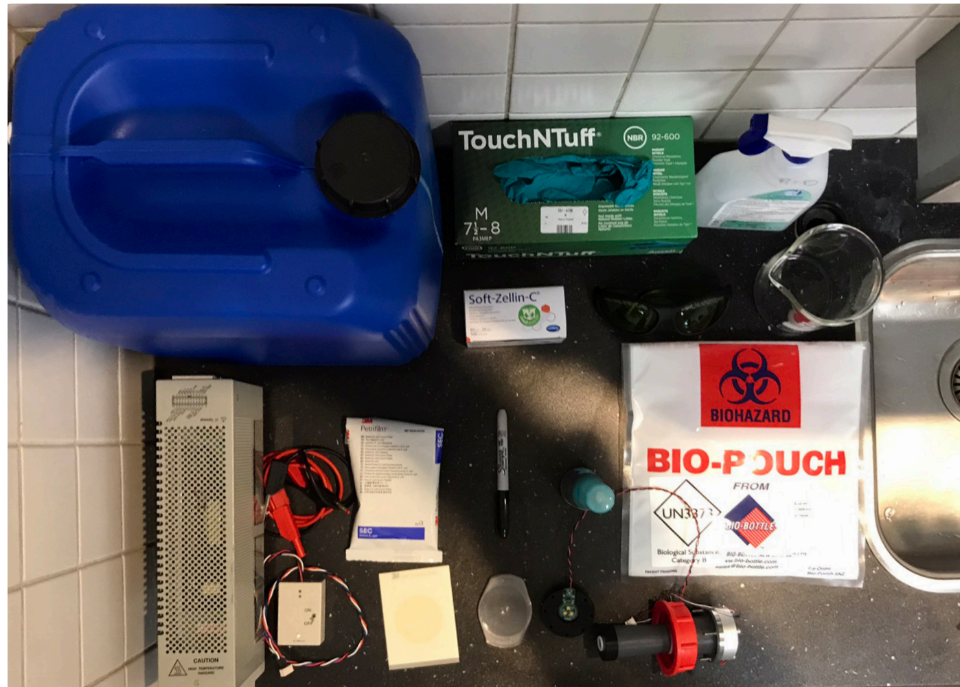
Figure 93: Overview of all the products used for the test. From LTR: power source, Petrifilm, jerrycan, water treatment products, disinfection wipes, gloves, UV-C protection glasses, E.coli sample, measuring cup.
