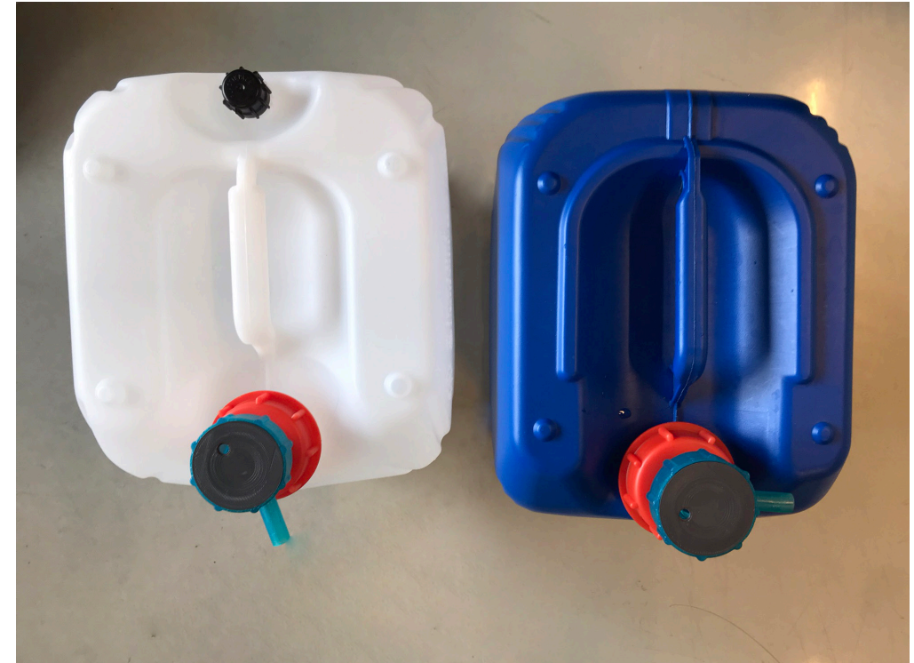
Figure 101: Two different jerrycans, with the same cap size, having different thread designs and affecting the spout alignment.
