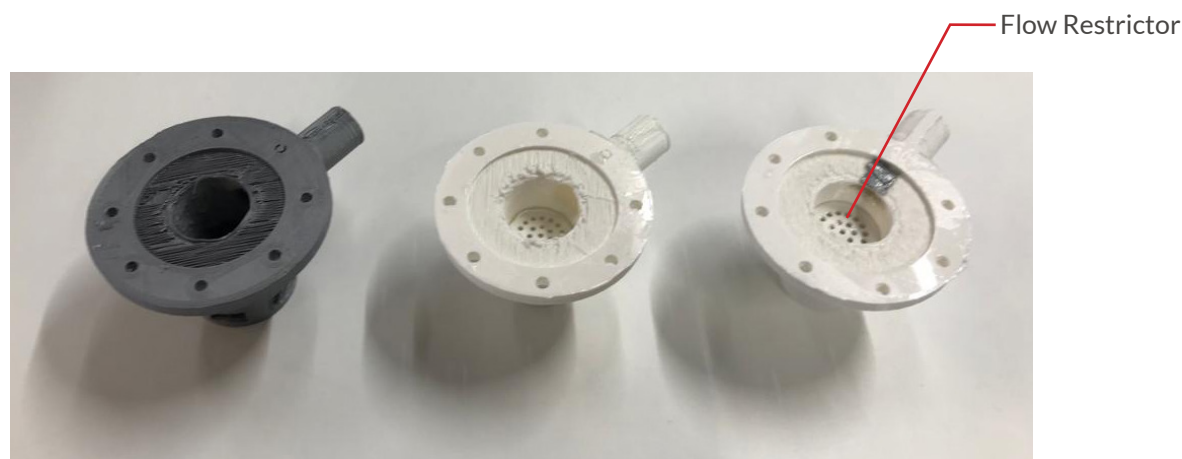
Figure 76: Different flow restrictor and tap designs.
