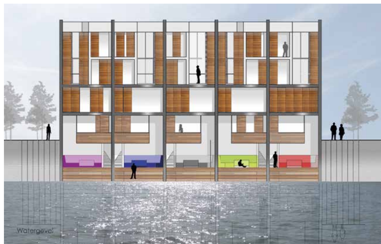
Figure 26. Facade view: Flood proof outdoor spaces seen from the riverside.
