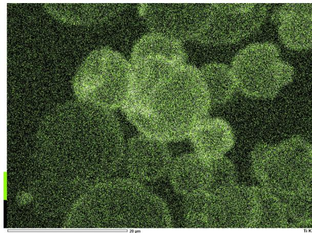
Figure 2.8 (b) EDS Elemental Mapping of  $\text{TiO}_2$ -coated Expancel
