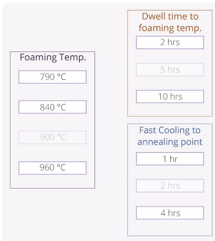
Figure 37. Parameters related to manufacturing process, foaming temperature-heating rate-cooling rate. To these, it should be added the dwelling time, which was not investigated thoroughly. Foaming temperature is always dependant on the main material used, as it should be defined according to the temperature of glass softening. Thus, this set of parameters describe the heating schedule for glass foaming, upon variant results can be achieved.
