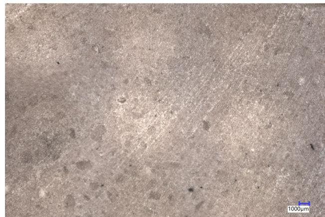
Figure 81. Cut and polished surface of sample TS10, microscopic image in stitching mode, Image Source: Own.
