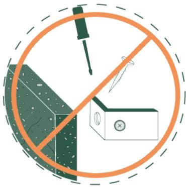
No direct screwing on the material
