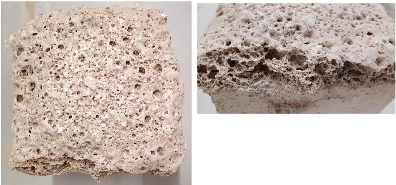
Figure 26. Photographs depicting the reacted sample of cement and aluminosilicate and its produced surface roughness and porosity.
