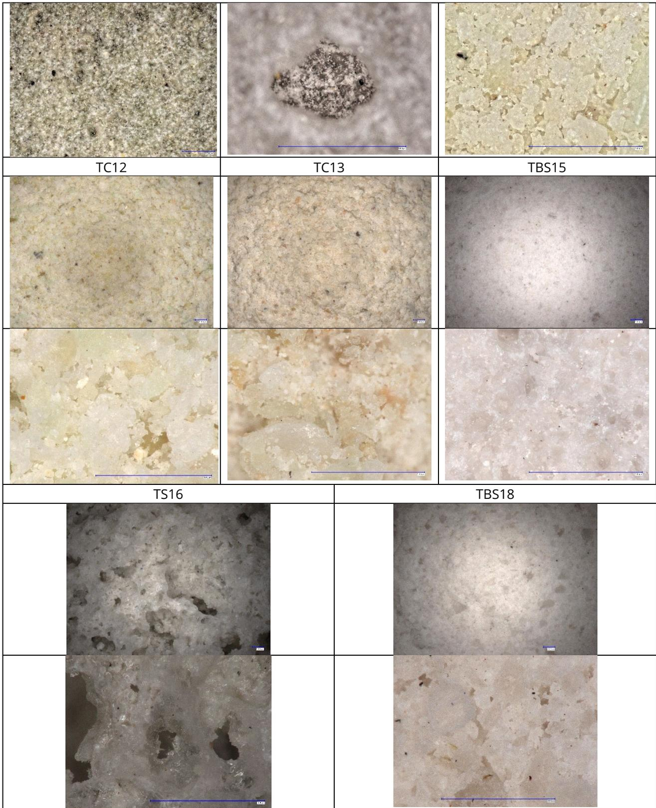
Appendix\_Table 3. Microscopical documentation of all the cubic samples produced for testing their porosity & hydraulic properties. Samples of a tile shape and the ones used for compressive strength were excluded from the image analysis of the digital microscope (VHX-7000 series, Keyence located at the Faculty of Architecture). Image Source: TC01-TS10: captured with the aid of T. Bristogianni, rest: Own.
