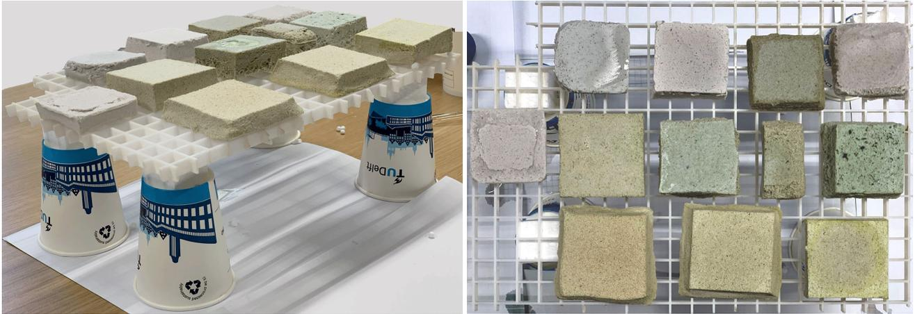
Figure 65. Experimental set-up to test how permeable is the microstructure, by dropping 1-5 ml of water onto the surface of the slated samples and measuring the time, while monitoring the effect of the results.
