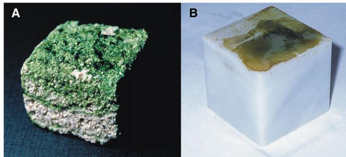
Figure 8. Photographs of experiments on primary bioreceptivity, showing the varying microorganism species promoted on the substrates' properties, affected mainly by surface roughness. From left to right: a) calcarenite, b) marble
