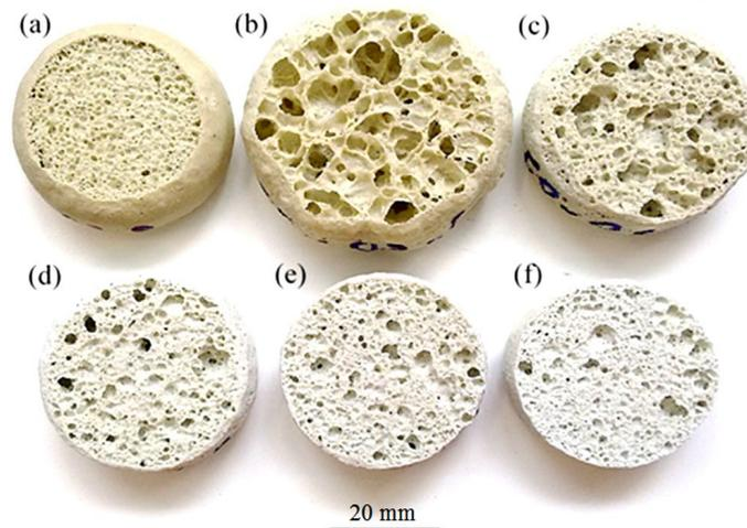
Figure 34. Image showing the porosity, foam expansion and dimensional changes of samples fires at 900 °C / 30 min with different content of eggshells in the mixture, (a) 1 wt%, (b) 3 wt%, (c) 6 wt%, (d) 9 wt%, 12 wt%, ( e) 15 wt% and (f) 30 wt%.
