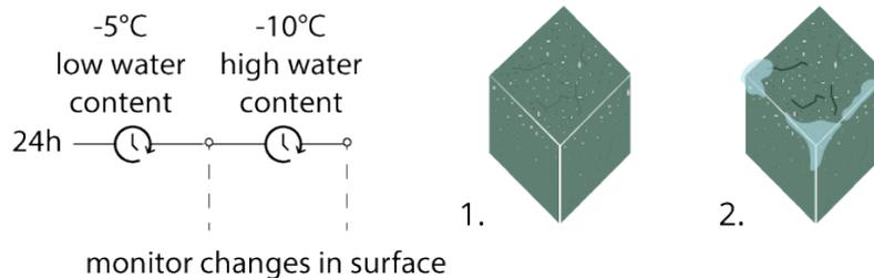
Figure 47. Alternative freezing conditions to test the material's resistance to frosting. These circles should be repeated more times to form an outcome according to material testing guidelines for market products.
