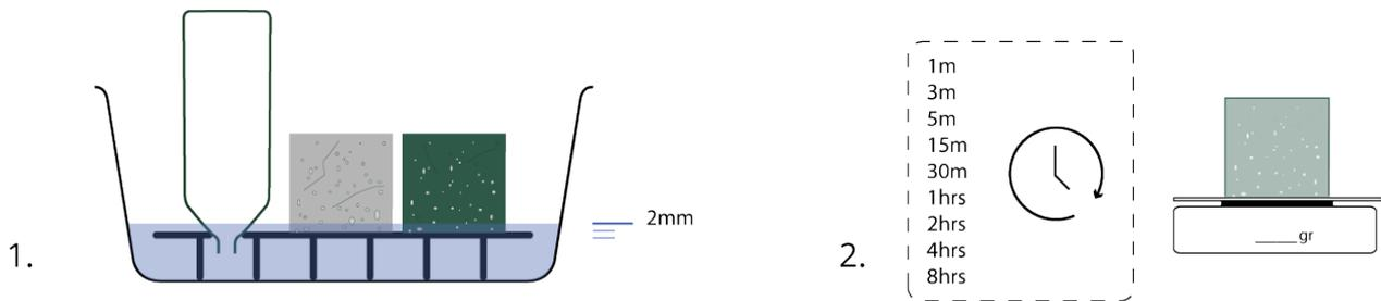
Figure 44. Diagram showing schematically the set-up for the absorption rate test and the time intervals for the measurements to determine the absorption curve.
