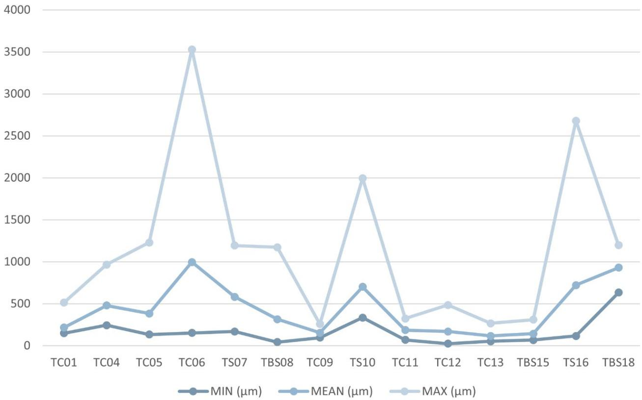
Chart 1. Lined-chart illustrating the pore sizes values of the polished surfaces of the cubic samples that were tested microscopically. Apart from the mean, the greatest range in sizes can be identified in the specimens TC06, TS10 and TS16, showing an uneven pore-distribution.
