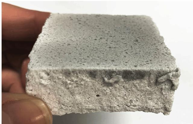
Figure 68. Photograph of sample TBS08, where the darker-coloured areas are moist from the dropped water, showing how permeable the material is.
