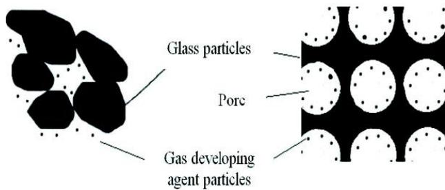
Figure 31. Diagram portraying how pores are formed from the initial state and during the sintering process of glass with the gas agent in the mixture. Pores are spherically depicted, for easier mathematical calculations that allow a 5% error instead of polygonal shapes that increase complexity.
