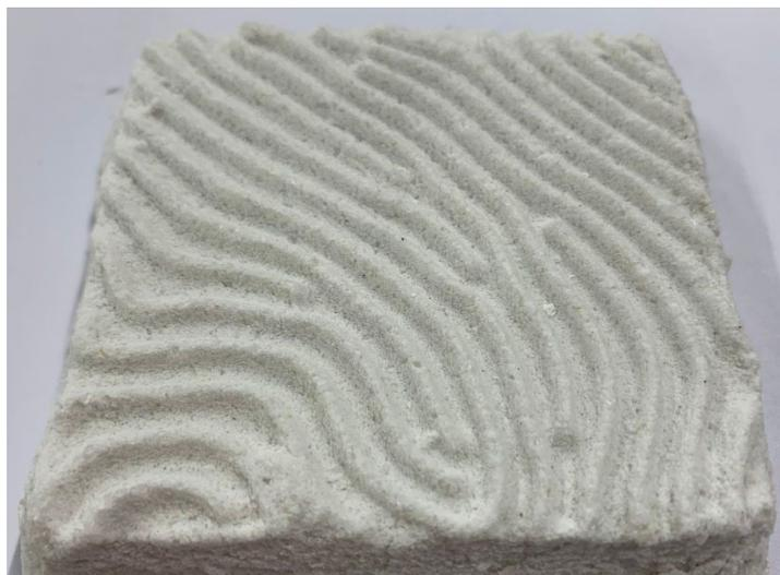
Figure 97. Sample TBS22 depicted to showcase the detail of the formed surface, in contact to the mould, to monitor the level of mould reaction. Image Source: Own.
