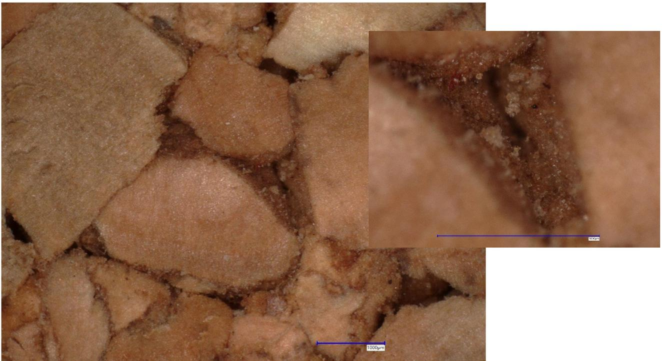
Appendix\_Figure 3. Microscopic image taken on 04/05/2022, from a kitchenware cork under investigation by Hartmann N. during Bucky lab course. As cork particles are bonded by its natural resin, produced under pressure, pores identified to be connected to the outer surface, are greatly affected by the particle size
