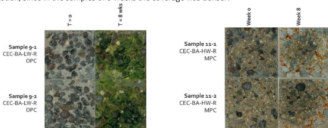
Figure 12. From left to right: a) Samples produced by Portland Cement and Crushed Expanded Clay, Bone Ash with low water/cement ratio showcasing high green coverage, while the observed microorganisms expanded partially also on top of altered the aggregate, b) Mixture with Magnesium Phosphate cement and Crushed Expanded Clay, Bone Ash with high water/cement ratio. Image Source: Fig. 8 & 9, pages 12-14, (Veeger et al., 2021).
