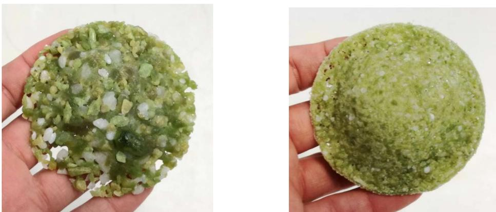
Figure 23. Photographs of the produced samples from different coloured glass bottles kiln-cast at 970 °C. From left to right: out of small shards and powder.
