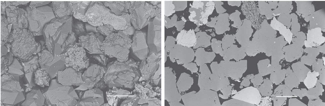
Appendix\_Figure 8. Clashach sandstone coarse structure in a fracture surface packaged grains of 0.2-0.5 mm in diameter electron micrographs by Francis Clegg.
