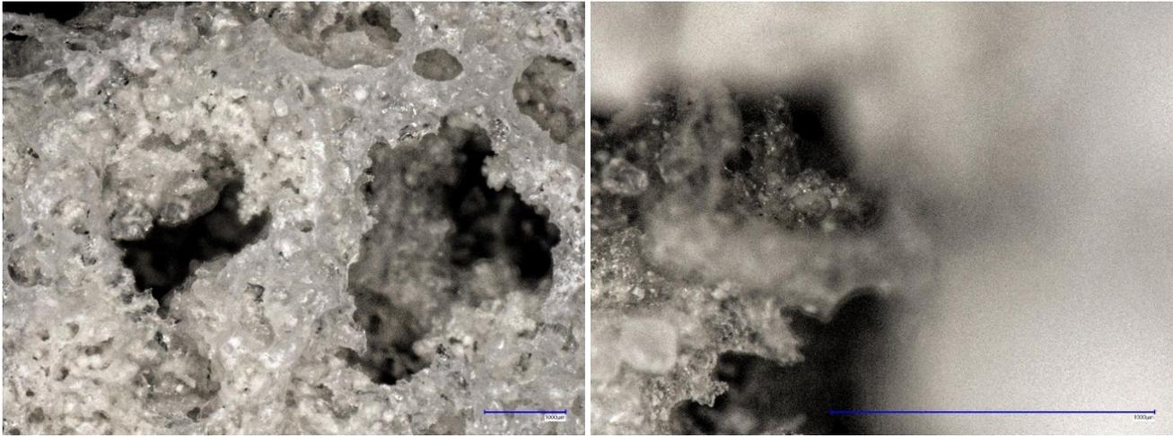
Figure 60. Microscopic images of TS16, at different zoom scales (x50 & x200), revealing the highly porous microstructure formed by the combination of Soda-lime powder & small-sized cullet, which was characterized by expansion during foaming at 840 °C, as seen in the Appendix\_Table 02. The resulted pore size range in this mixture was phenomenally large compared to the rest of the samples, mainly due to the expansion effect.
