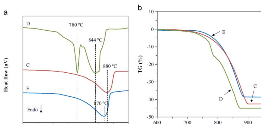
Figure 29. Thermal analysis curves of foaming agents: (a) DTA and (b) TGA, D: domolite, C: Calcite, E: Eggshells, Image Source: Fig.1, Fernandes et al., 2014.
