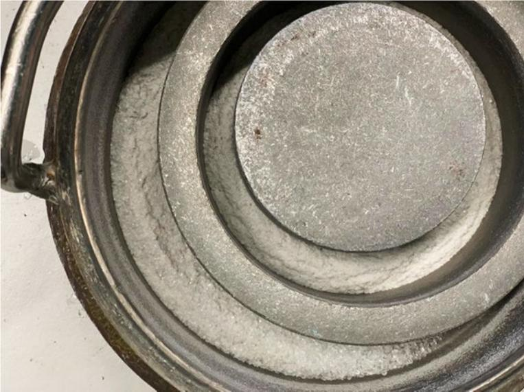
Figure 39. Soda-lime crushed cullet turned to powder after 4sec of sieving (Herzog Disk Mill).
