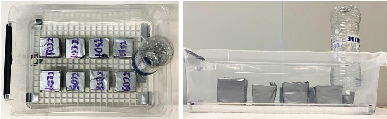
Figure 74. Experimental set-up for testing the water absorption rate. Image Source: Own (29/04/2022).
