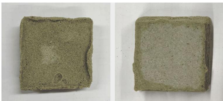
Figure 70. Dispersion effect along the surrounding sides of the sample TC09, implying that its vertical network is not fully permeable.
