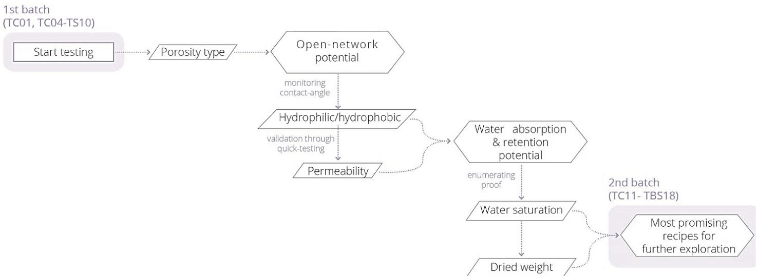
Figure 72. Flowchart illustrating the testing process as a methodology for choosing the parameters to be tested (Ingredients – Temperature – Heating schedule). Results from quick testing are used as an input for the next experimentations, while the rest of the testing process continues for validation and further exploration.
