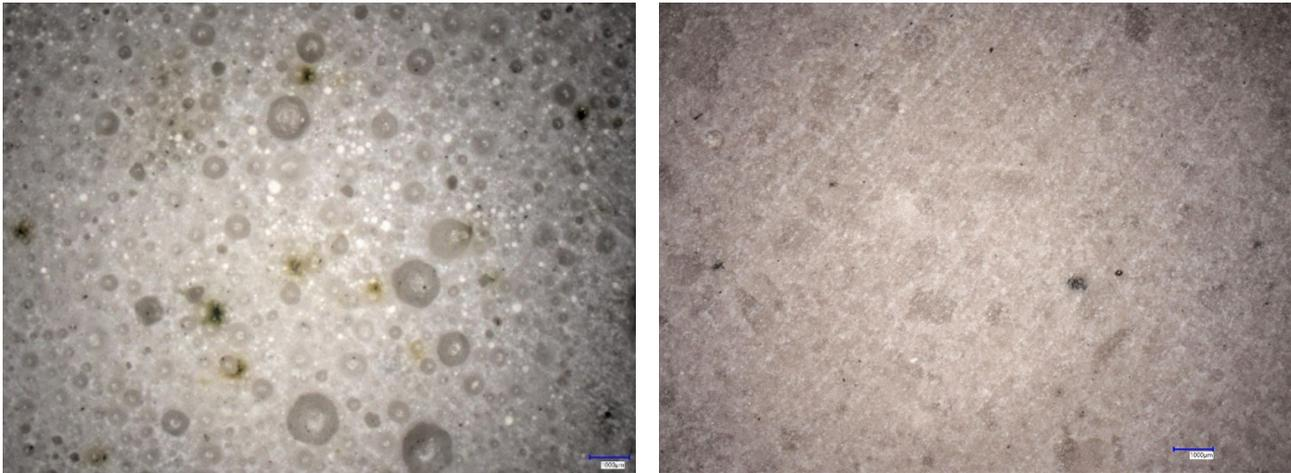
Figure 53. Microscopic images of samples TS07 & TS10, illustrating the two different images of closed porosity represented in Type 01. Images were captured with zoom x20, blue line representing the scale equals with 1000µm.
