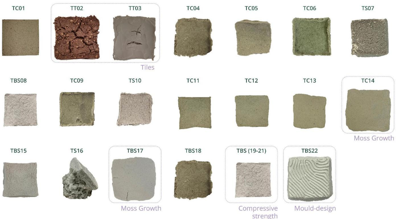
Figure 38. Overview of the produced samples analysed in Table 5.
