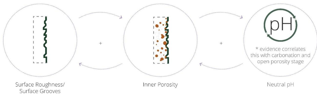
Figure 4. Diagram illustrating material conditions for bioreceptivity. Image Source: Own.
