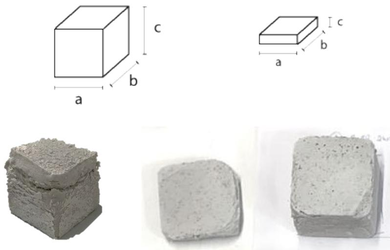
Figure 40. (from left to right) The original moulded shape, and the two shapes obtained after the cut.
