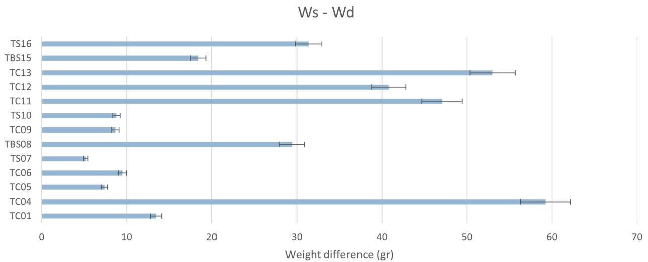
Chart 2. Comparative analysis of the saturation level of the cubic-shaped samples.
