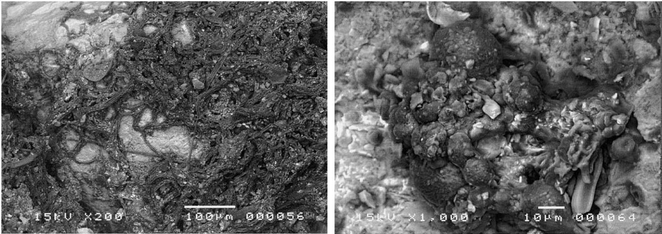
Figure 11. From left to right: a) Image produced by SEM micrograph representing Chlorophyceae on concrete forming a green stain x1000, b) LVSEM micrograph zooming in the black stain formed by Cyanophyceae x1000. Image Source: Fig 5 & 3, page 3 (Dubosc et al., 2001).
