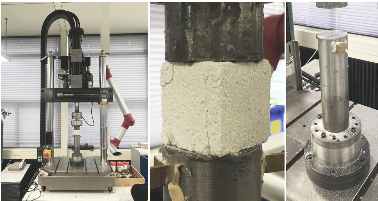
Figure 76. (from left to right) a) Compressive strength test set-up, b) cracks of permanent deformation appeared in the specimen TBS21 under the maximum load of 3,14 kN, c) apparent material residue after testing. Image Source: Own.
