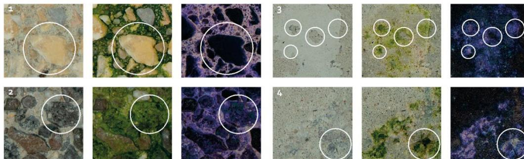
Figure 7. Images of the tested specimens for bio-growth, showing increased green coverage on those that a surface retarded was used. In contrast to the ones that biofilm grew only on surface imperfections or broken corners.
