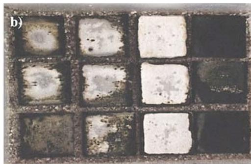
Figure 20. Experiment set-up in horizontal surfaces. Specimens were positioned on top of a vermiculite layer to reassured that all the needed nutrients together with the water content were provided.
