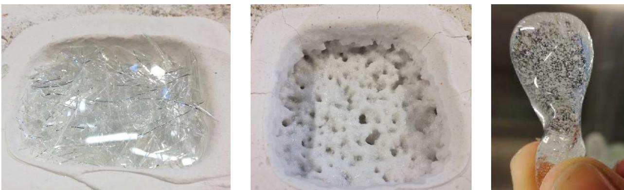
Figure 22. Images showing the different steps of Alkali-aluminosilicate glass treated, being retrieved from a mobile phone screen. From left to right, before tested, fired at 1250°C and at 1500°C.
