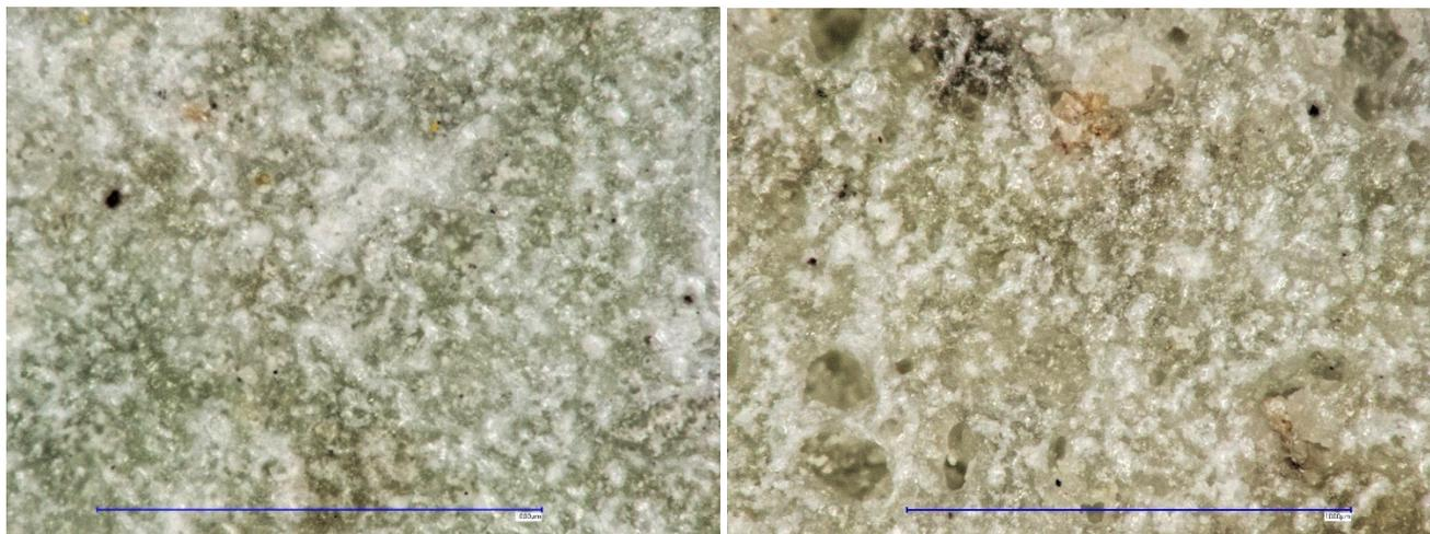
Figure 56. Microscopic images of TC01 & TC05, at the larger zoom x200 in the digital microscope (VHX-7000 series, Keyence located at the Faculty of Architecture), showcasing the crystallized parts of the mixture together with other various ingredients represented with different colours and textures. The effect of foaming agent is evident from the existence of distinctive pore formations of larger sizes in the right image of TC05.
