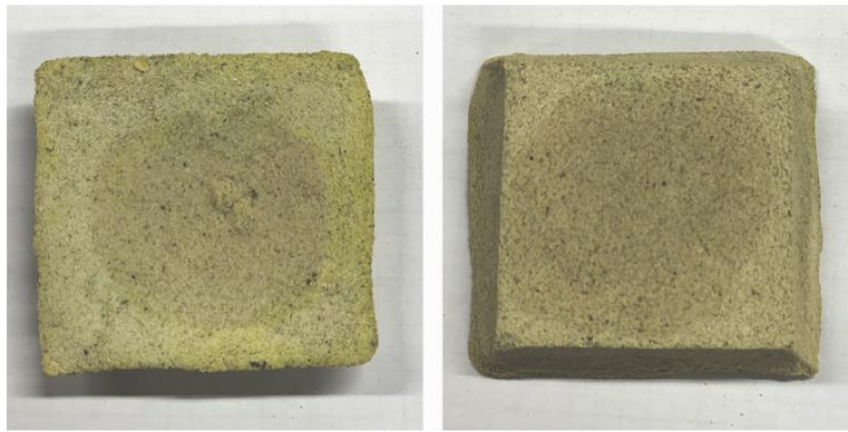
Figure 67. Photographs of sample TC12, made from Cyclon mix together with 5%wt of CaCO<sub>3</sub>, depicting the corrosion from water only on the surface which also has reacted with the mould. However, the water in comparison with sample TC13 has slightly limited dispersion.
