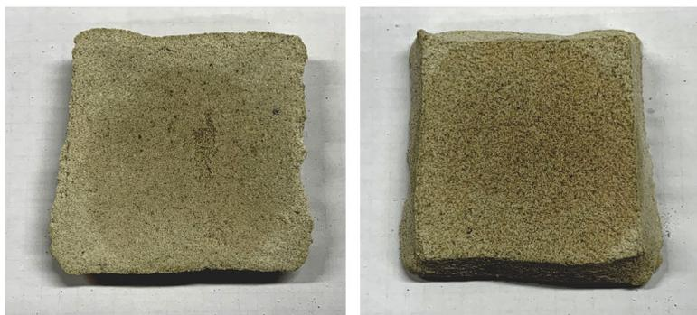
Figure 66. Photographs of sample TC13, a Cyclon mix with 10%wt  $\text{CaCO}_3$ , showing the stain of the dispersed absorbed water from the polished surface towards the opposite one.
