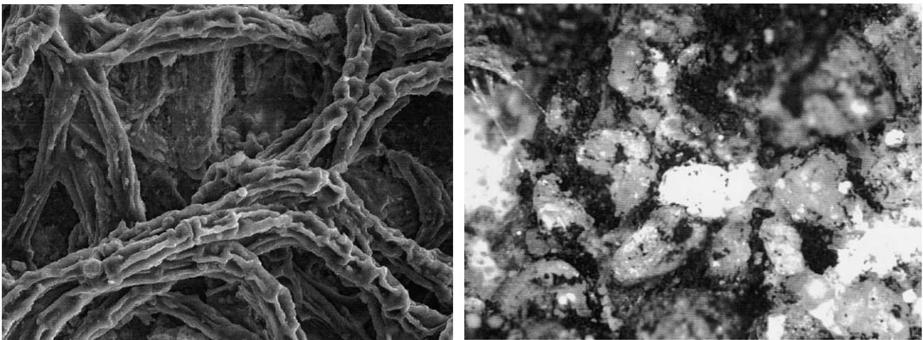
Figure 10. From left to right: a) LVSEM micrograph zooming in the green stain x200, b) Video-microscope micrograph of the black stain x100. Image Source: Fig 4 & 2, page 3 (Dubosc et al., 2001).
