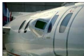
Figure 2. External mirror assembly for forward-looking LiDAR applications.
