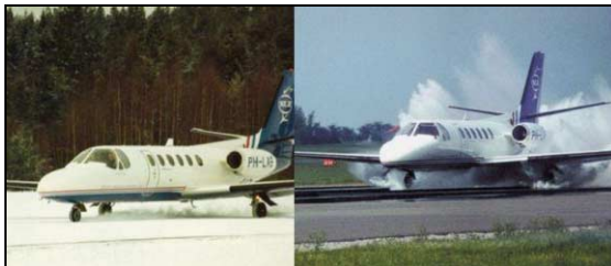
Figure 4. Take-off and landing trials on wet and contaminated runways.
