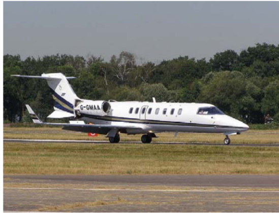
Fig 7. Delta fin configuration underneath the tail on a Learjet 45
