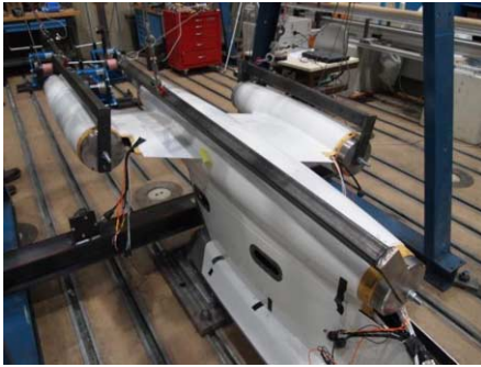
Figure 8. HALO Setup for static load test for DLR HALO PMS-Carrier.
