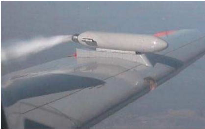
Figure 6. VFW 614, ATTAS upper wing smoke generator, DLR.
