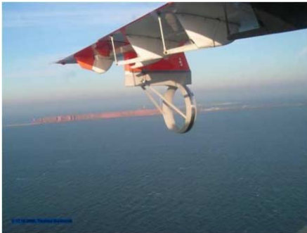
Figure 9. Antenna system mounted to DO228 wing.
