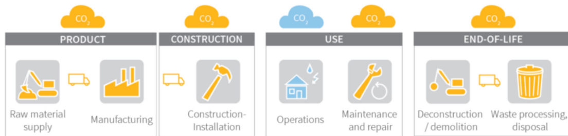
Figure 1.1. Embodied Carbon (yellow) and operational carbon (blue) across building life cycle. (Carbon Leadership Forum, 2020)
