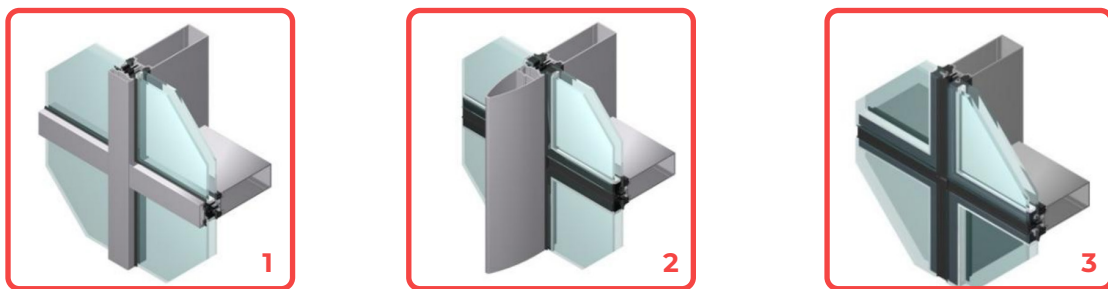
Figure 3.13. Three main applications of curtain wall system: (1) Standard continuous glazing, (2) Semi-structural glazing and (3) Structural glazing. (Kim, 2013)
