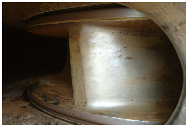
Figure 3.10: Blade Exit after pumping 11.000 TDS
