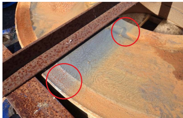
Figure 3.4: Wear Plate after pumping 11.000 TDS
