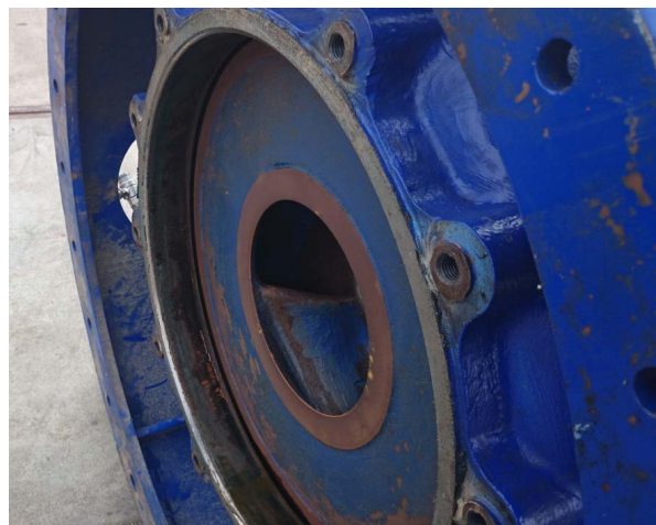
Figure 3.12: Suction Shroud after pumping 0 TDS
