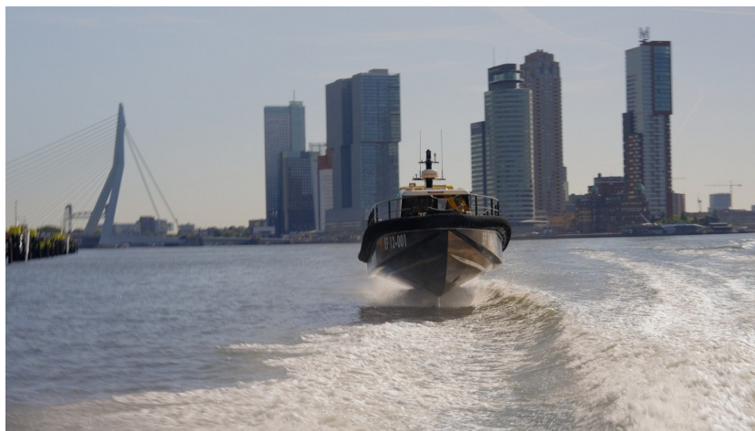
Figure 2.3: The foiling Artemis EF-12 patrol vessel operating on the Nieuwe Maas river in Rotterdam (Artemis Technologies, n.d.)
